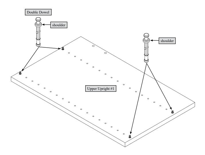
Insert four Double Dowels completely into the holes in the Upper Upright #1.
