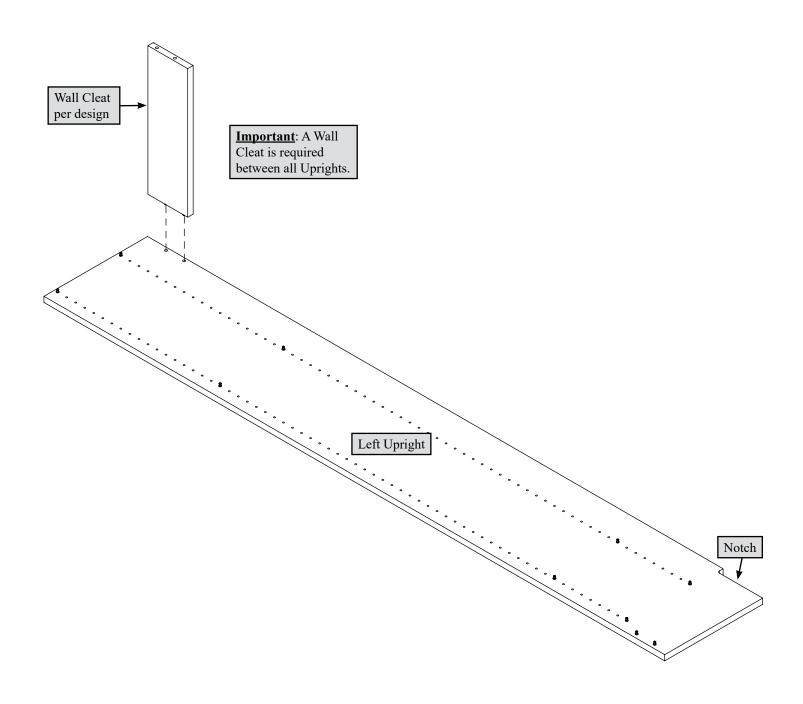
Wall Cleats come with pre-glue dowels in them. Fasten a Wall Cleat to the Left Upright by pushing the wood dowels in the Wall Cleat into the Upright.
