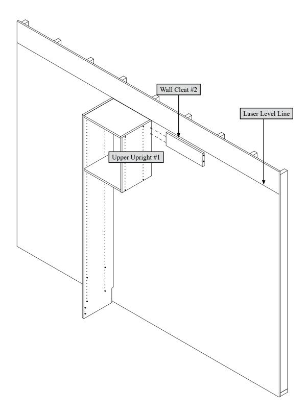
Wall Cleats come with pre-glue dowels in them. Fasten a Wall Cleat to Upper Upright #1 by pushing the wood dowels in the Wall Cleat into the Upright.
