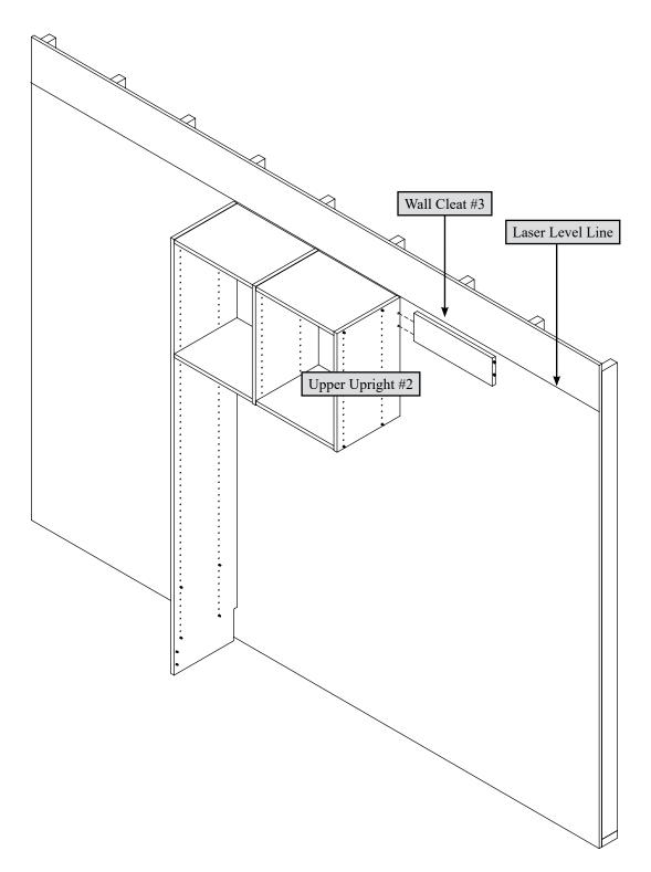
Wall Cleats come with pre-glue dowels in them. Fasten a Wall Cleat to Upper Upright #2 by pushing the wood dowels in the Wall Cleat into the Upright.
