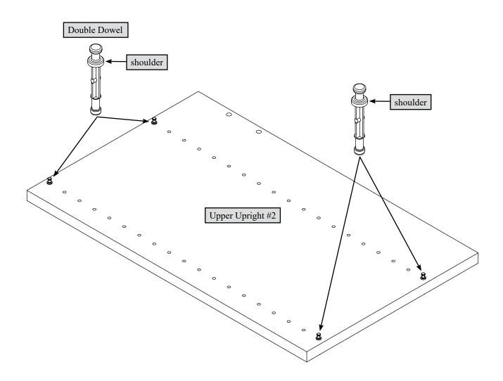
Insert four Double Dowels completely into the holes in the Upper Upright #2.
