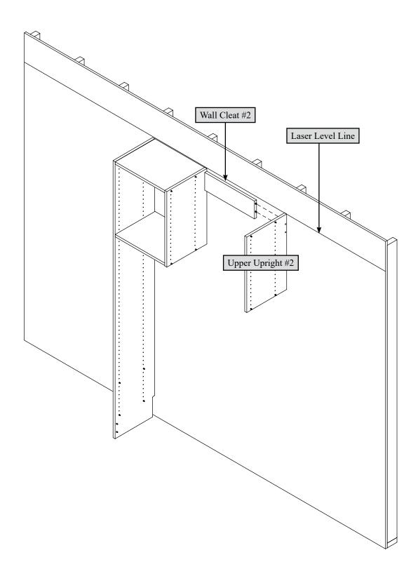
Push the Upper Upright #2 onto the wood dowels in Wall Cleat #2.
