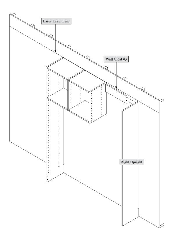
Push the Right Upright onto the wood dowels in Wall Cleat #3.
