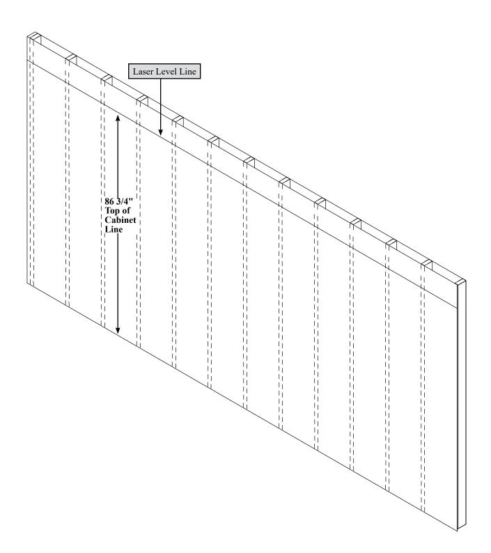
With a level or laser, create a line 86 3/4" off the floor onto your wall to indicate the top edge of the Left Upright.
