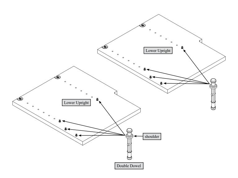
Push eight Double Dowels into the exact holes how in the Lower Uprights.
