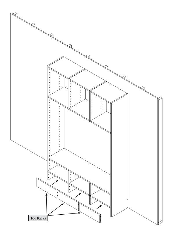
Push the upper connectors in the Toe Kicks onto the upper Push-In Dowels and Double Dowels. Next, rotate the Toe Kick on the upper Dowels until the connectors are exposed. Tighten two upper connectors in each Toe Kick. Rotate the Toe Kicks down completely onto the lower Double Dowel.
