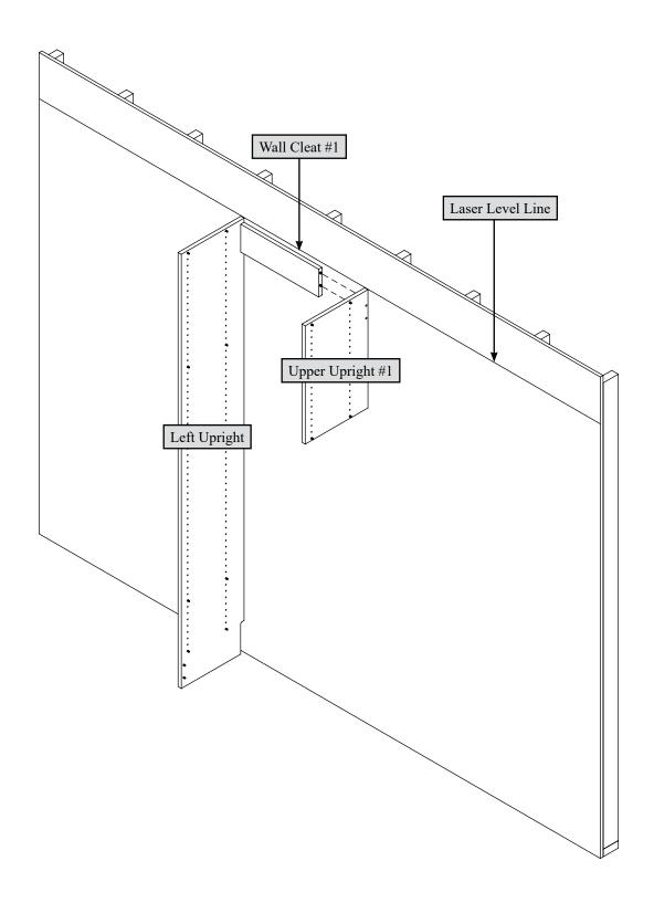
Push the Upper Upright #1 onto the wood dowels in Wall Cleat #1.
