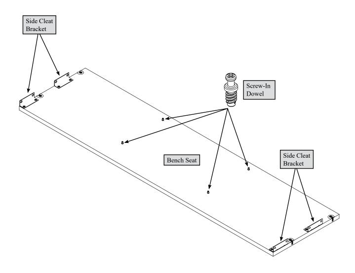
Fasten the Side Cleat Brackets to the Bench Seat with eight 9/16" Wafer Head Screws.
