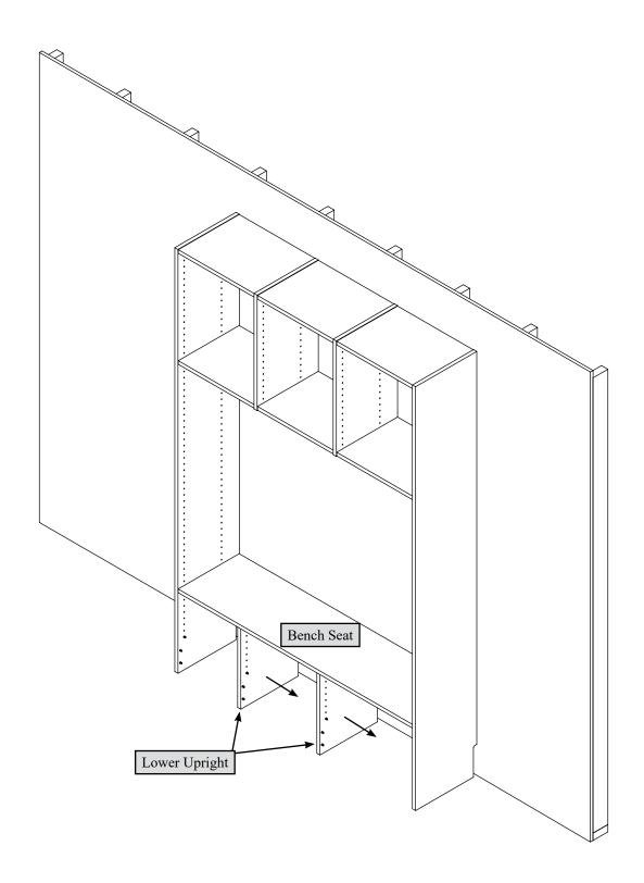
Fasten the Lower Uprights to the Bench Seat. Tighten four Connectors.
