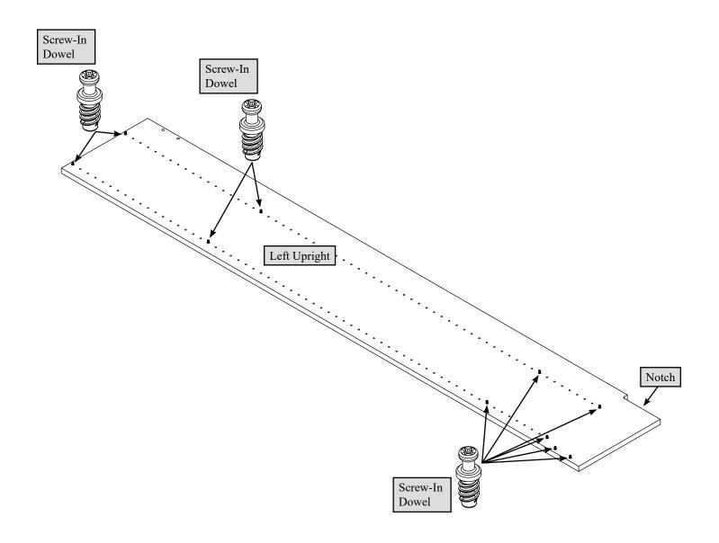
Turn ten Screw-in Dowels into the exact holes shown in the Left Upright.
