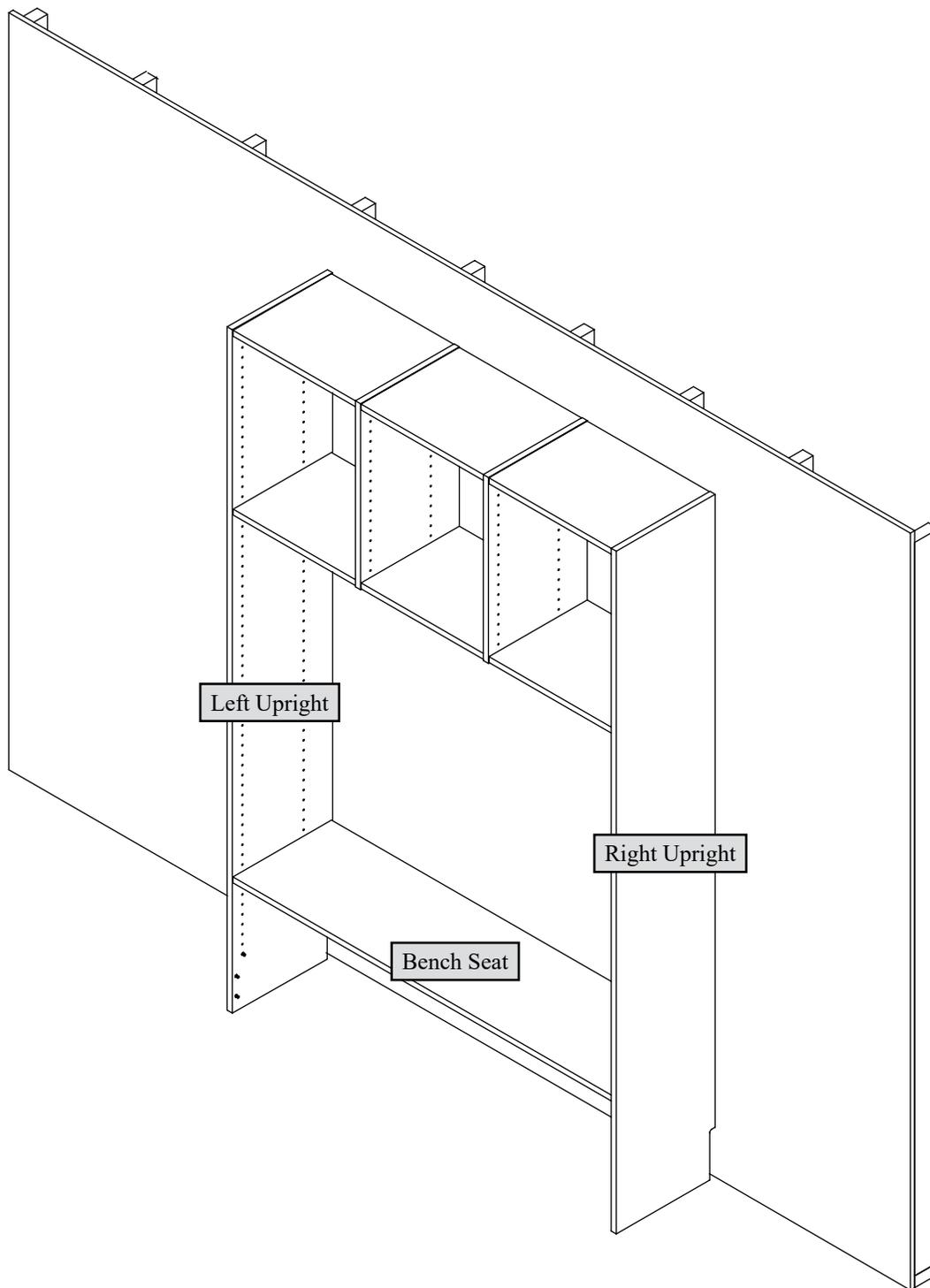
Fasten the Bench Seat to the Left and Right Uprights. Tighten four Connectors.
