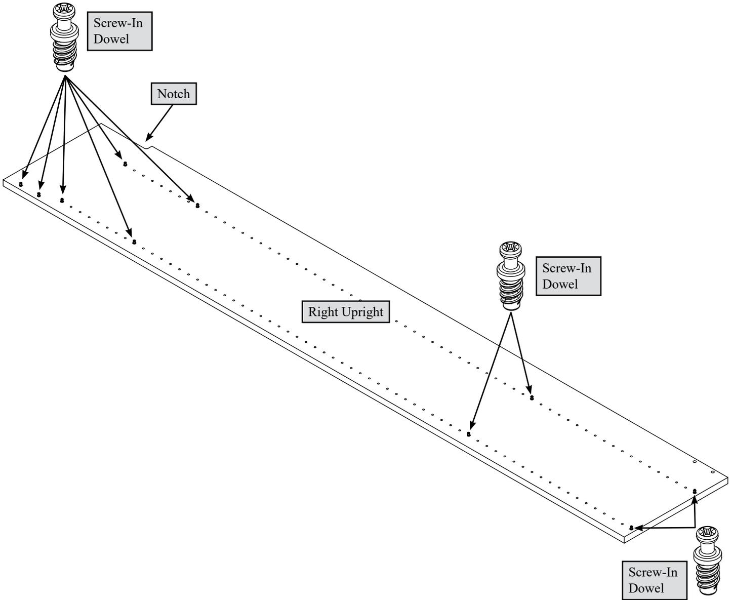
Turn ten Screw-in Dowels into exact holes shown in the Right Upright.
