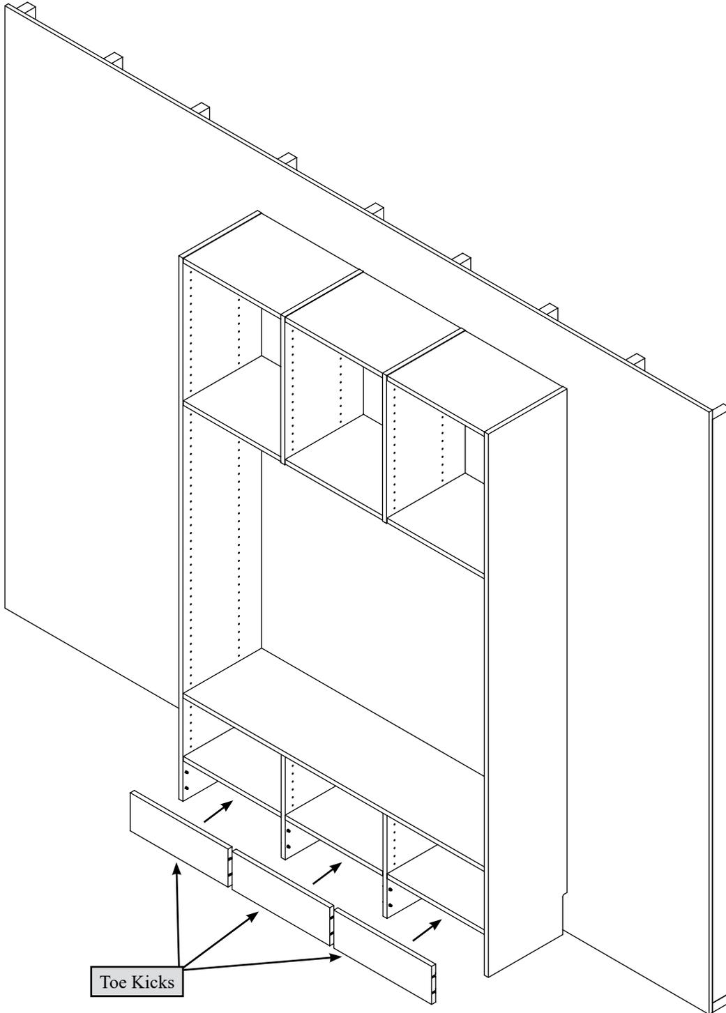
Push the upper connectors in the Toe Kicks onto the upper Push-In Dowels and Double Dowels. Next, rotate the Toe Kick on the upper Dowels until the connectors are exposed. Tighten two upper connectors in each Toe Kick. Rotate the Toe Kicks down completely onto the lower Double Dowel.
