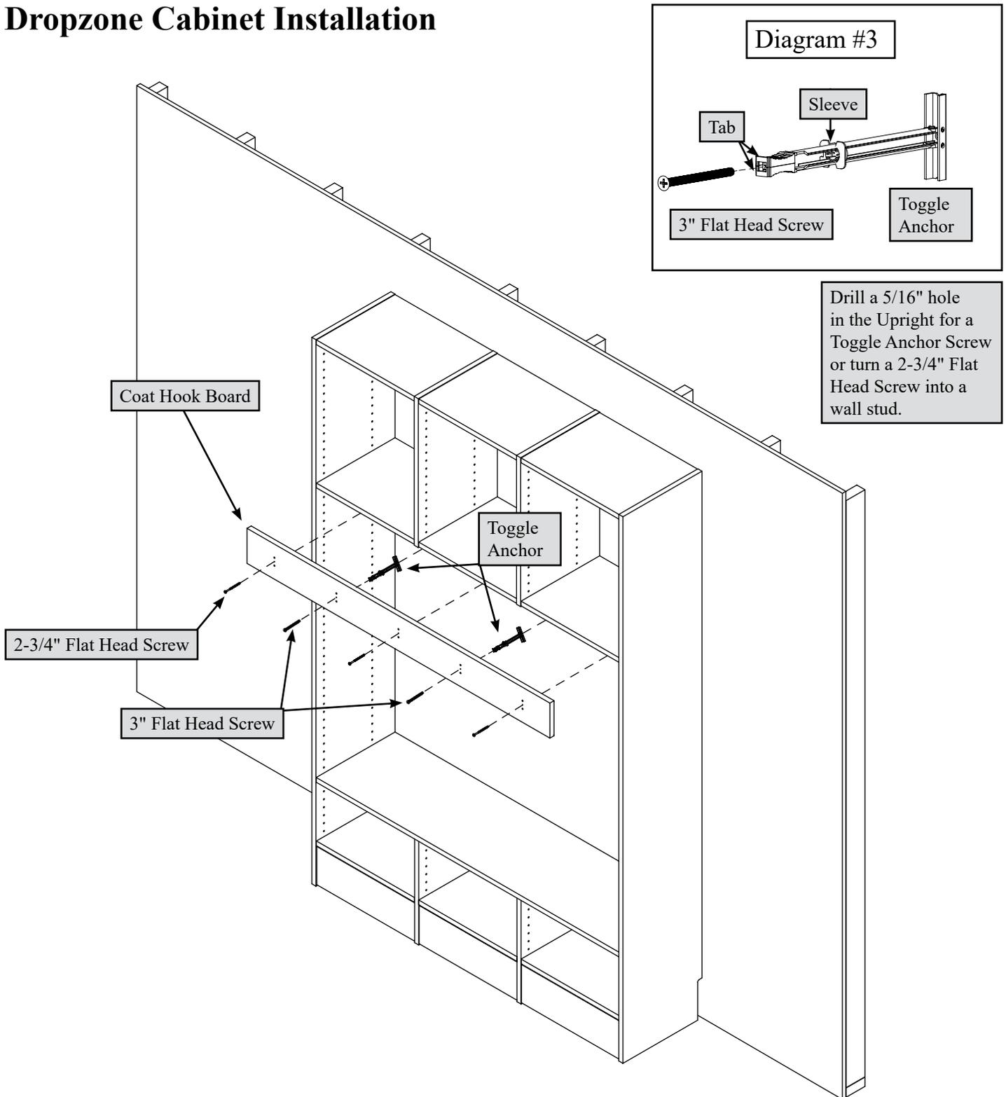
**IMPORTANT:** Fasten the Coat Hook Board to a wall stud with a 2-3/4" Flat Head Screw or with a Toggle Anchor if a wall stud is not available.
