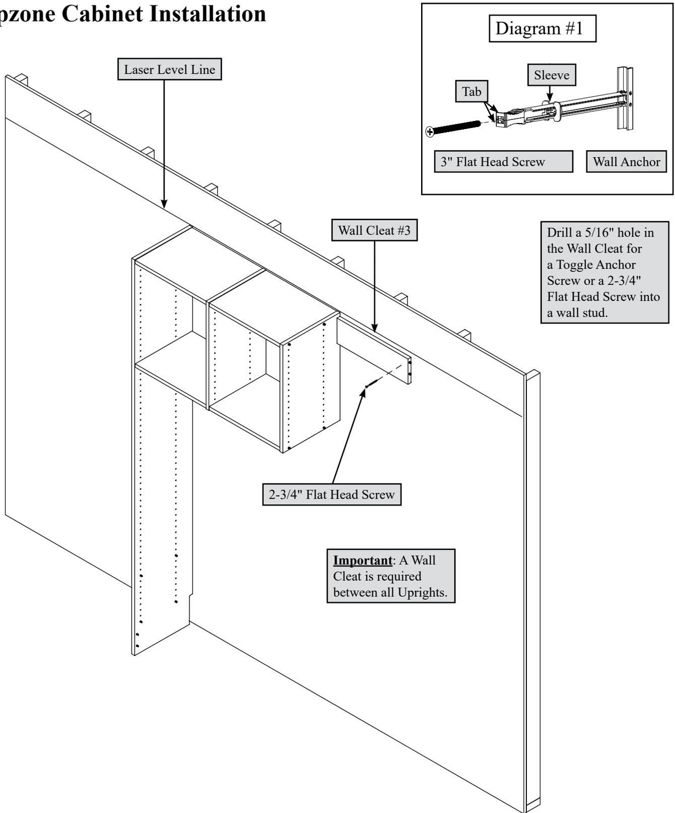
**IMPORTANT:** Fasten Wall Cleat #3 to a wall stud with a 2-3/4" Flat Head Screw or with a Toggle Anchor if a wall stud is not available.
