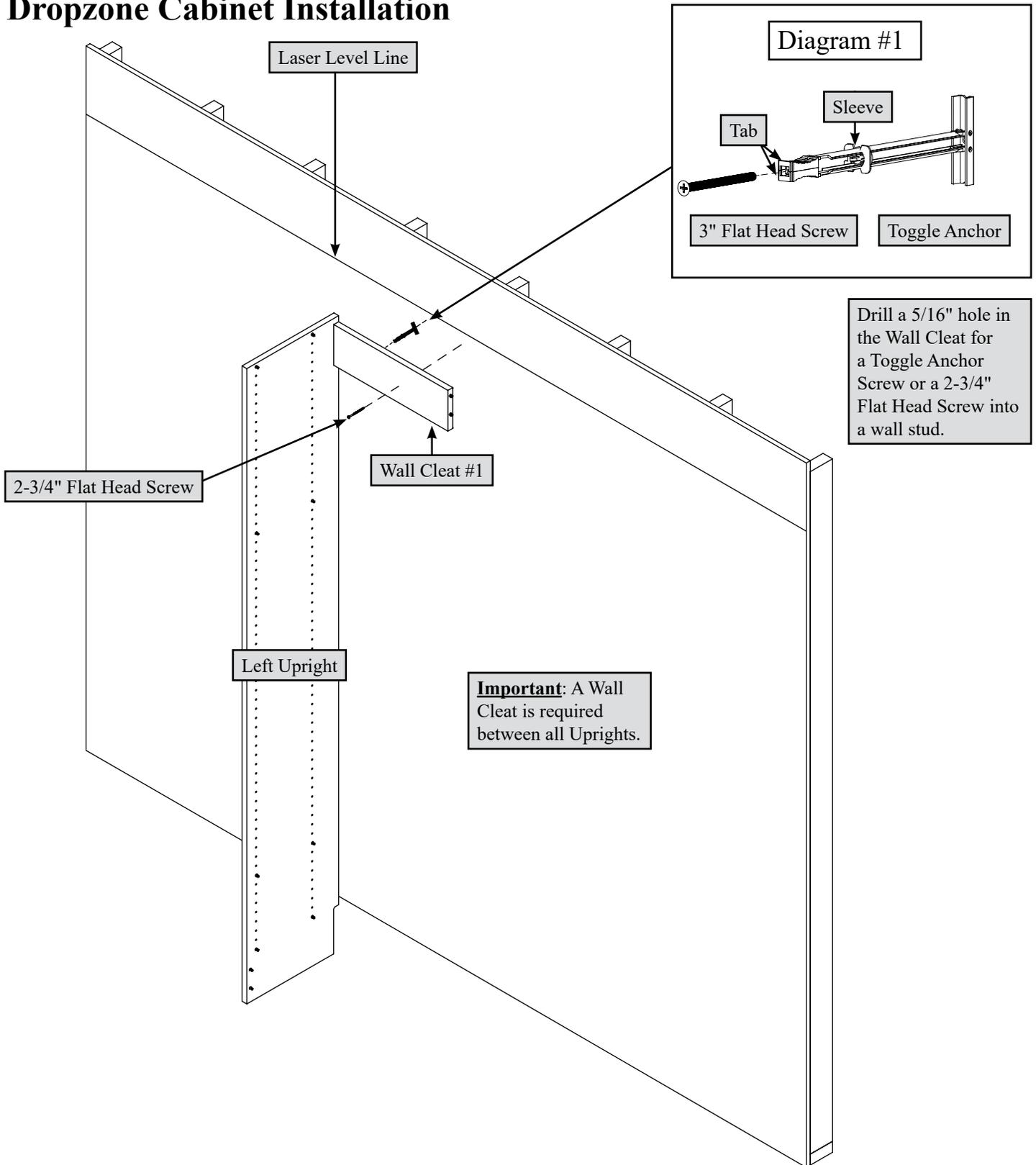
**IMPORTANT:** Fasten Wall Cleat #1 to a wall stud with a 2-3/4" Flat Head Screw or with a Toggle Anchor if a wall stud is not available.
