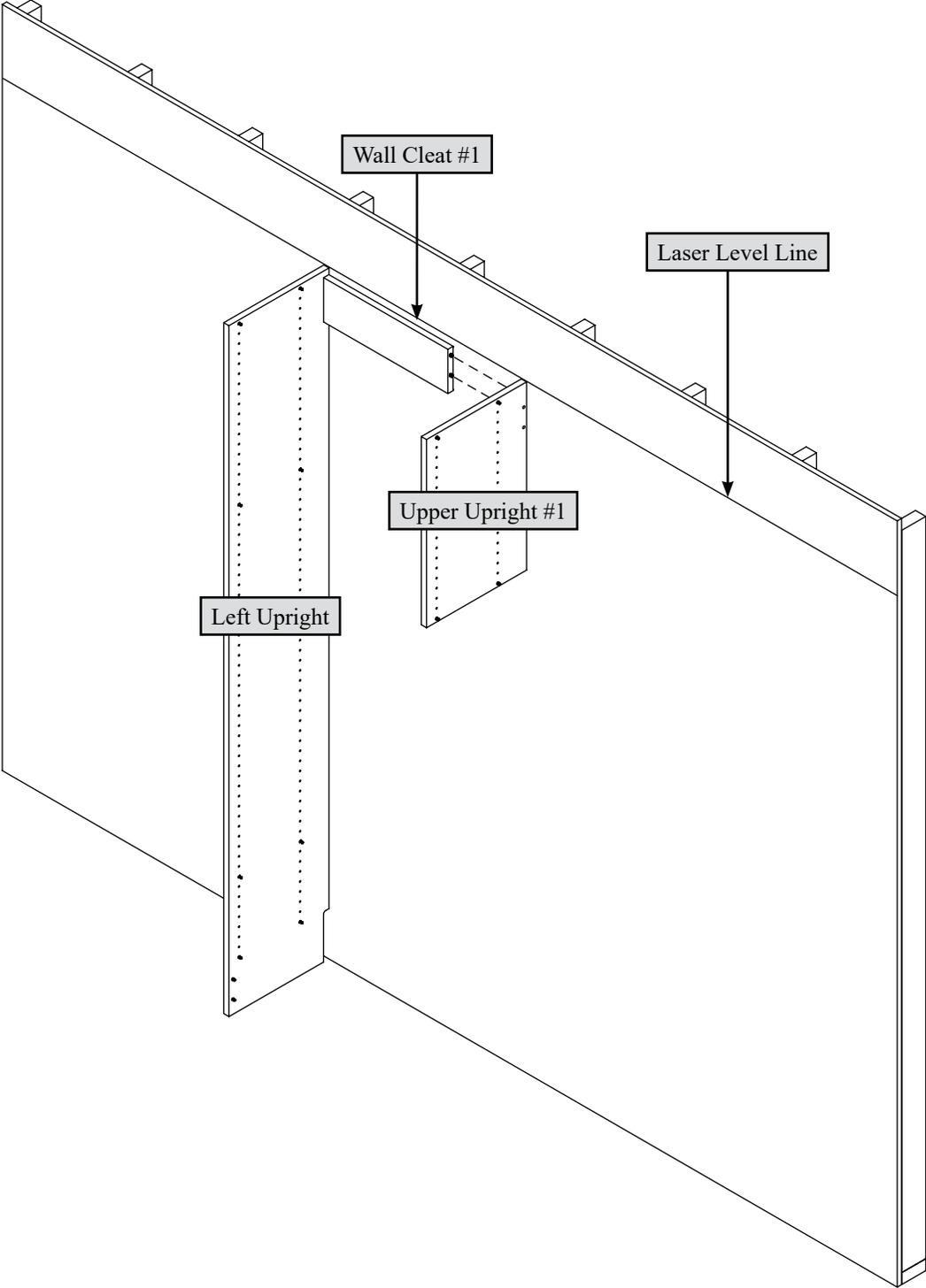
Push the Upper Upright #1 onto the wood dowels in Wall Cleat #1.
