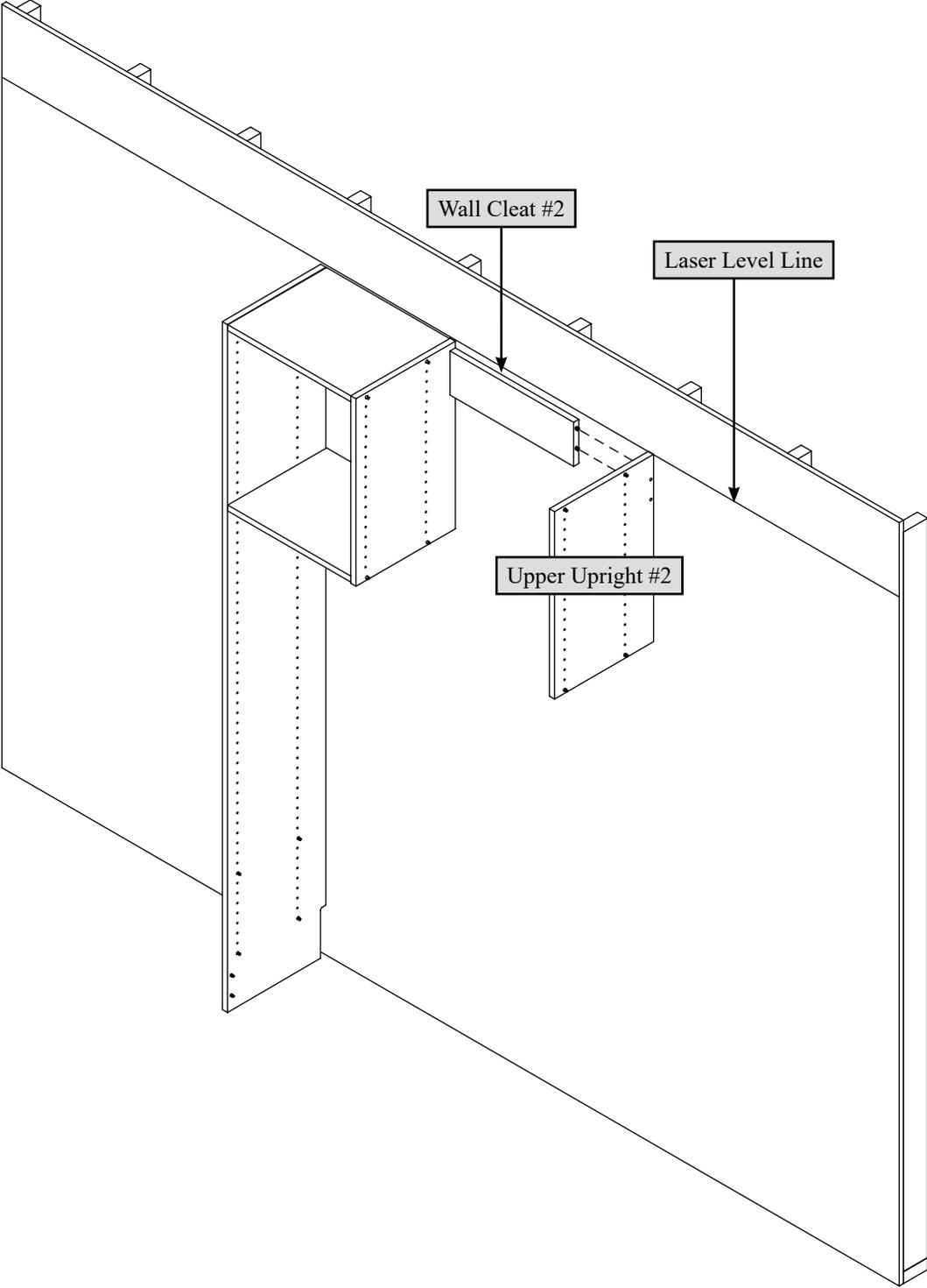
Push the Upper Upright #2 onto the wood dowels in Wall Cleat #2.
