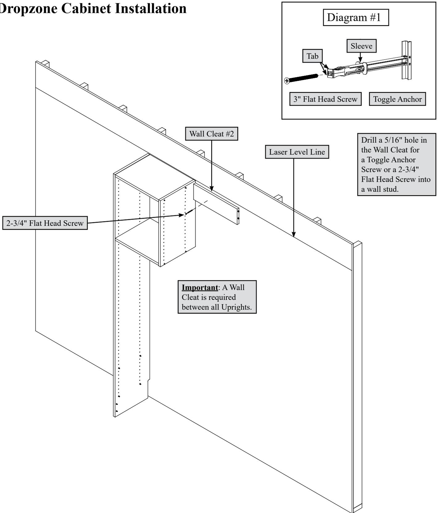
**IMPORTANT:** Fasten Wall Cleat #2 to a wall stud with a 2-3/4" Flat Head Screw or with a Toggle Anchor if a wall stud is not available.
