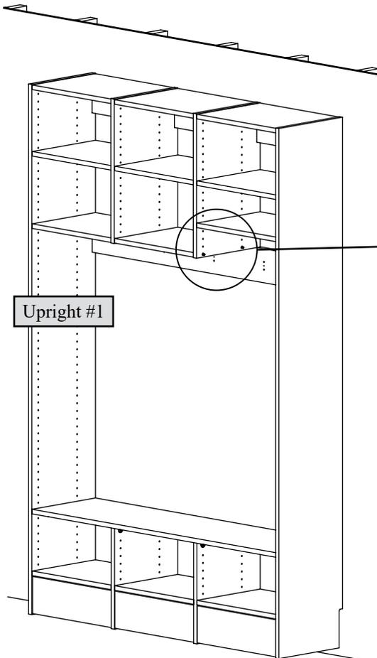
A Double Dowel is required in the exact orientation between two Fixed shelves that are horizontally in-line.
