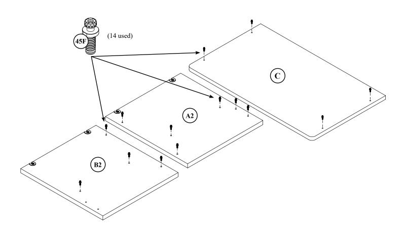
Push fourteen CONNECTOR DOWELS into the exact holes shown in the ENDS (A2 and B2) and TOP (C) until the shoulder of each CONNECTOR DOWEL restsW on the surface of the ENDS and TOP.
