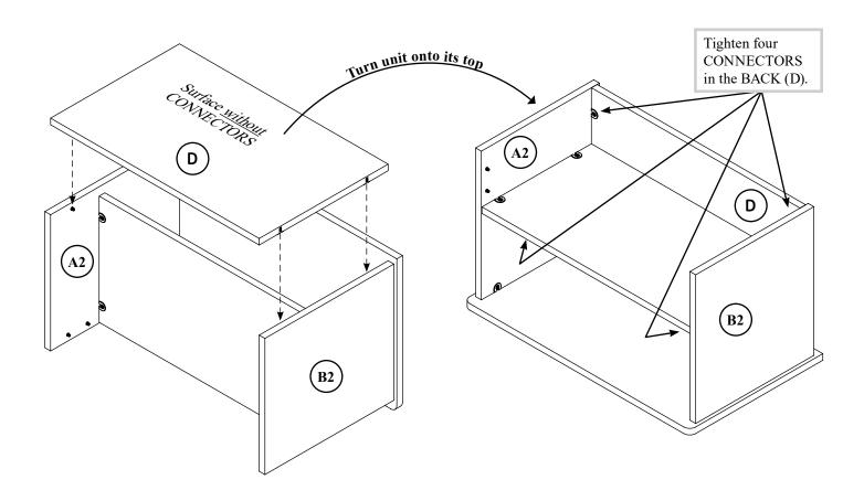
Place the CONNECTORS in the BACK (D) onto the CONNECTOR DOWELS in the ENDS (A2 and B2). Carefully turn your unit onto its TOP. Tighten four CONNECTORS in the BACK (D).
