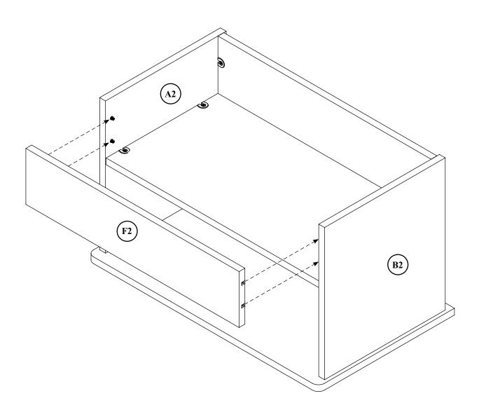
Push the TOE KICK (F2) onto the CONNECTORS in the ENDS(A2 and B2). Tighten four CONNECTORS.
