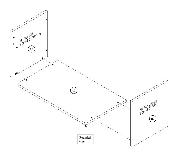
Fasten the ENDS (A2 and B2) to the TOP (C). Tighten four CONNECTORS.
