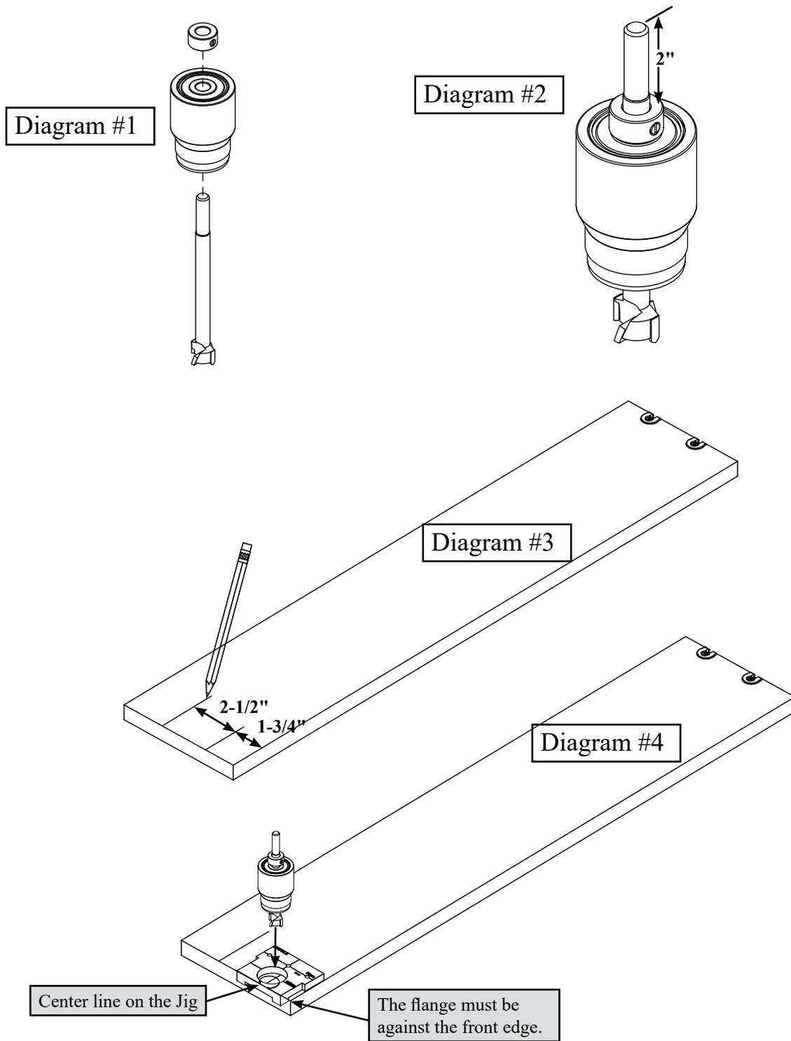
In some Designs, you may need to cut a Fixed Shelf to length and rebores holes to replace the connectors in the Shelf. Follow the diagrams and steps below for instructions.
