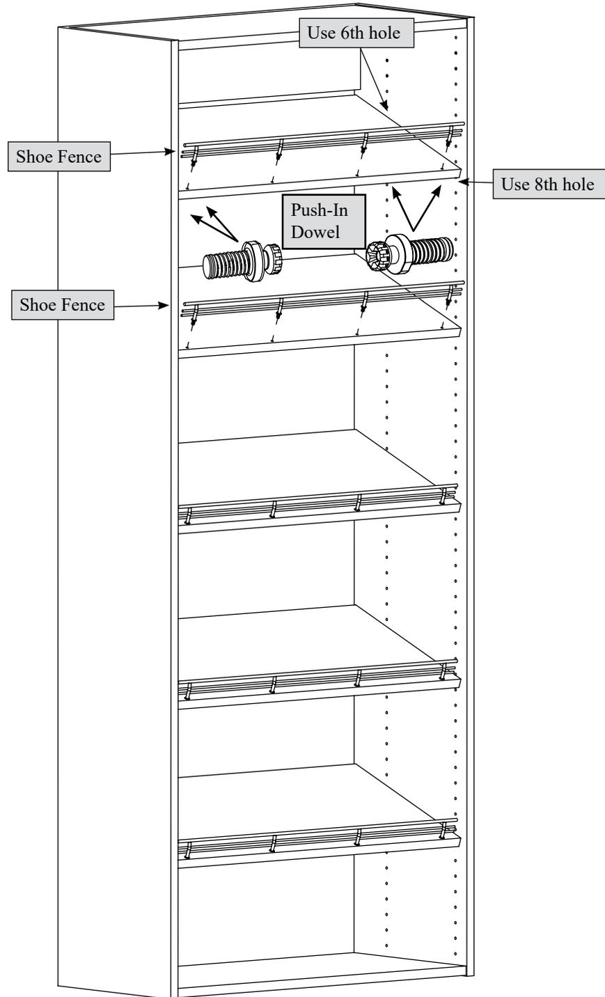
When locating a Shoe shelf in a Floor Cabinet, insert two Push-In Dowels into the 6th Upright holes below the top Fixed Shelf along the back edge.
