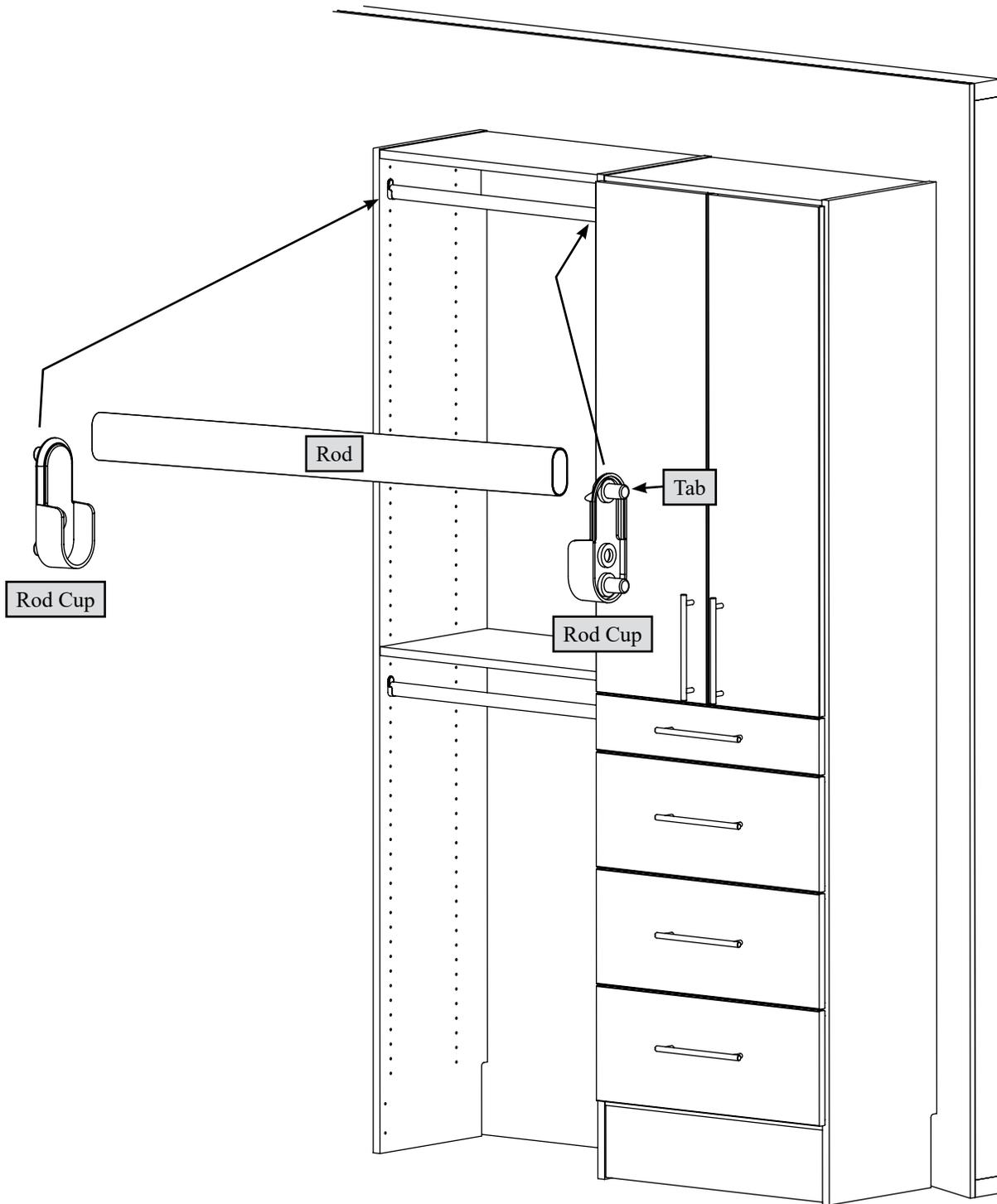
Insert the tabs of the Rod Cups into the exact holes shown.
