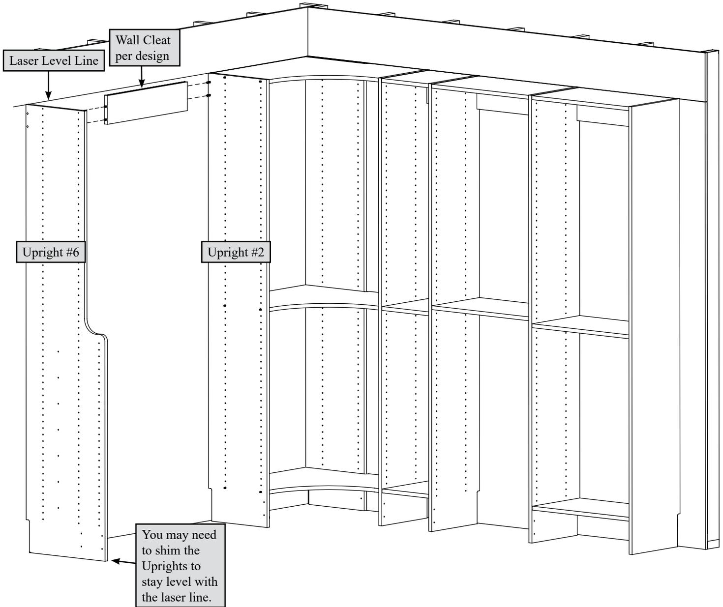
Fasten the Wall Cleat to the Uprights by pushing the wood dowels in the Wall Cleat into Uprights #2 and #6.
