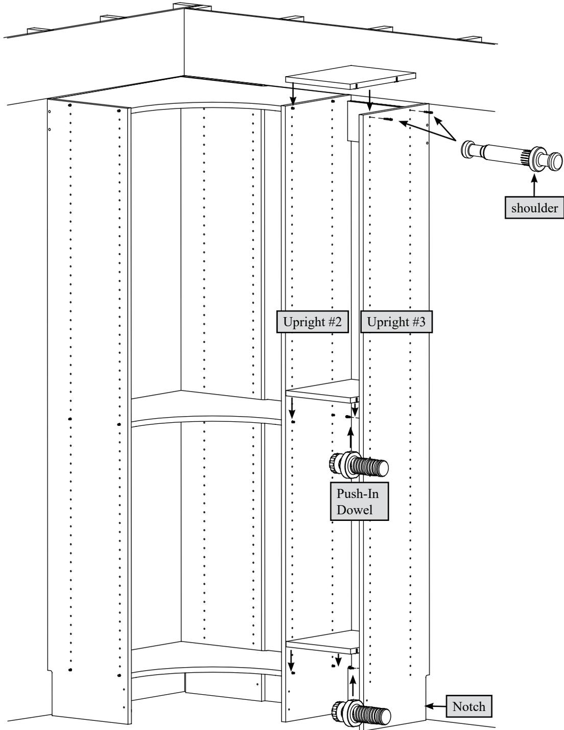
Insert two Double Dowels completely into the holes in Upright #3.
