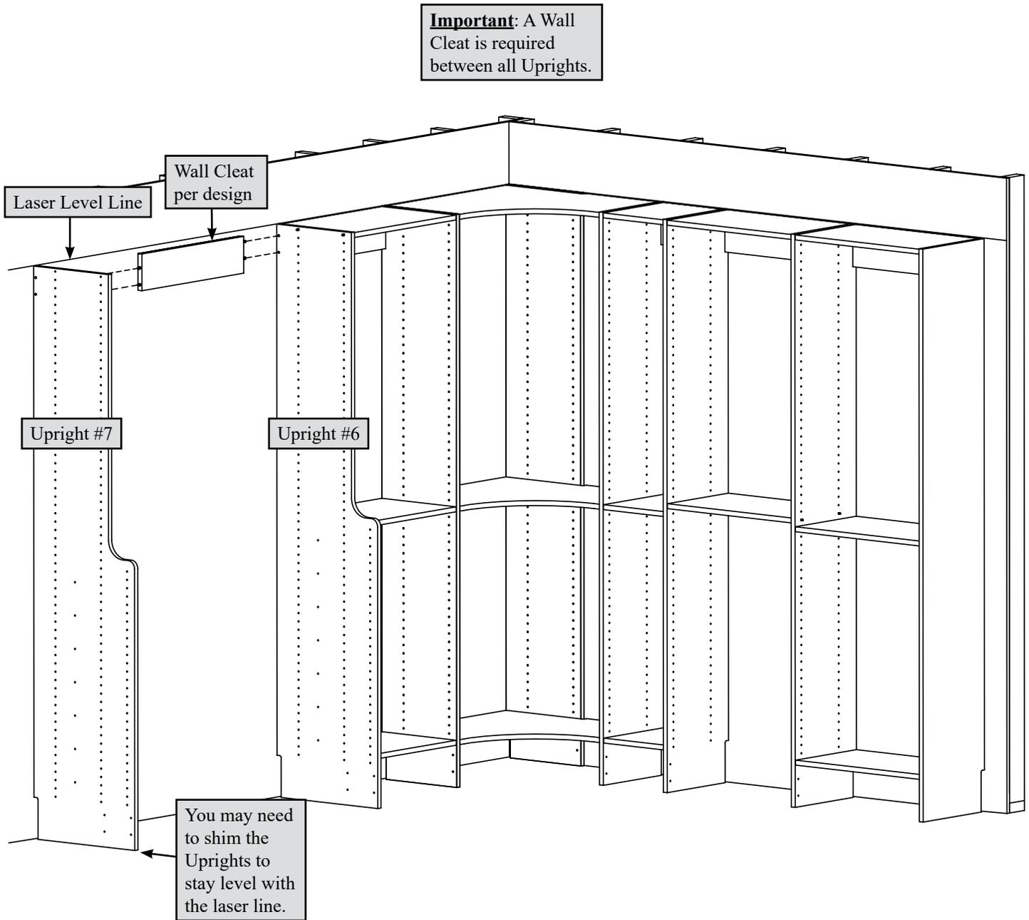
Fasten the Wall Cleat to the Uprights by pushing the wood dowels in the Wall Cleat into Uprights #6 and #7.
