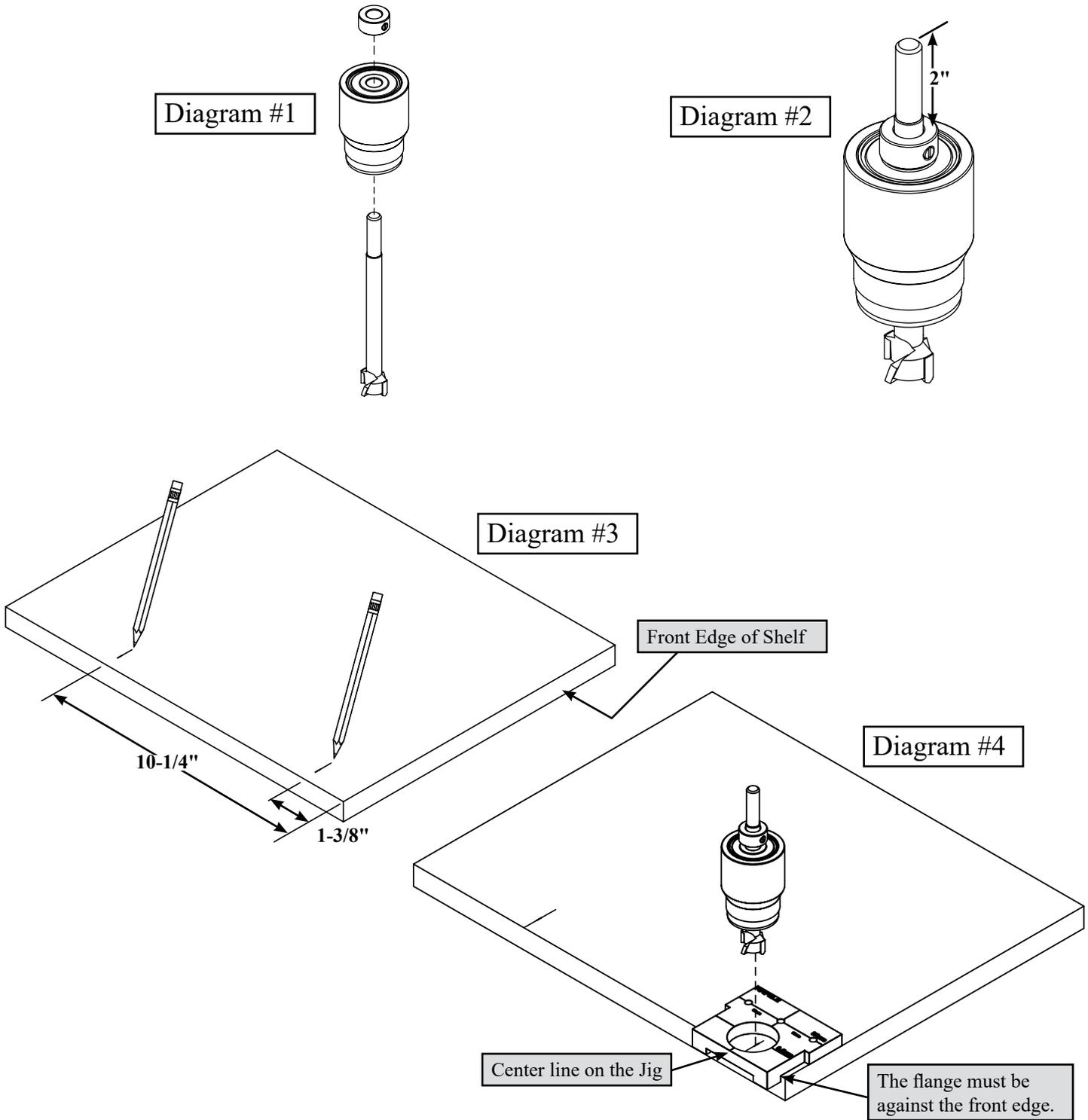
In some Designs, you may need to cut a Fixed Shelf to length and rebores holes to replace the connector holes in the Fixed Shelf. Follow the diagrams and steps below for instructions.
