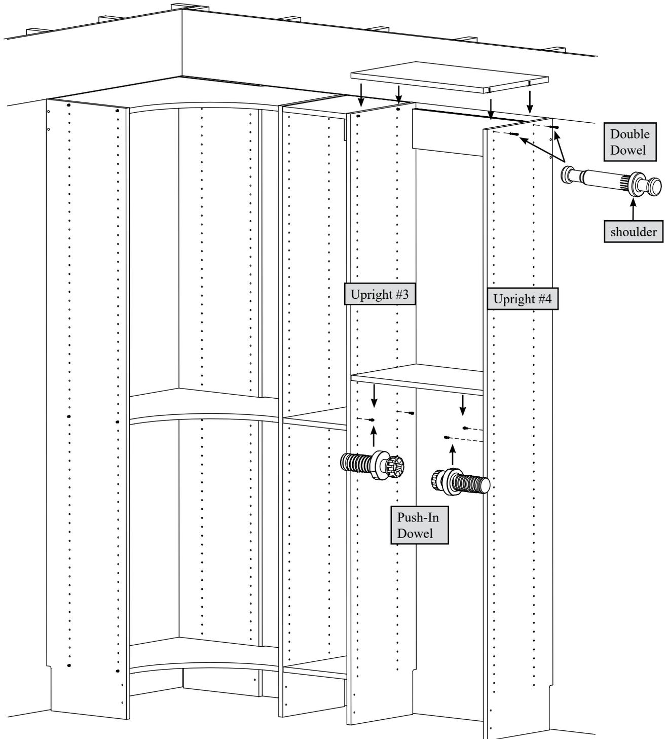
Insert two Double Dowels completely into the holes in Upright #4.
