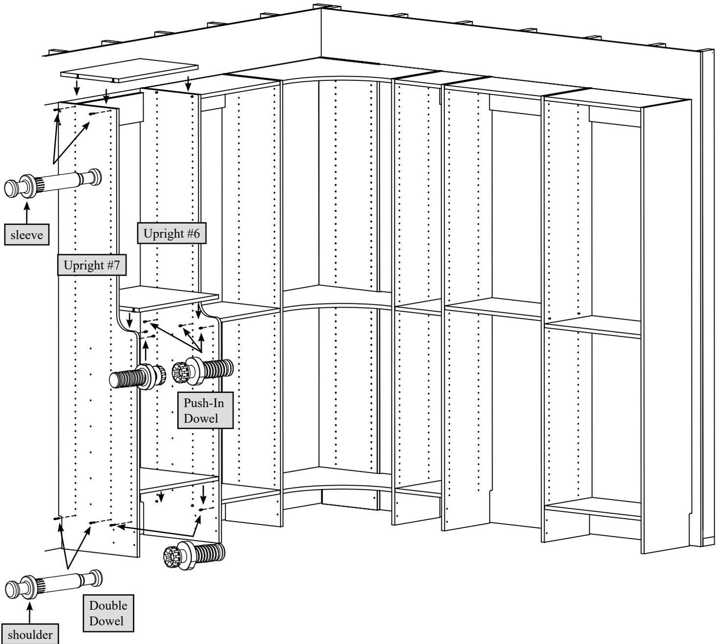
Insert four Double Dowels completely into the holes in the Upright #7.
