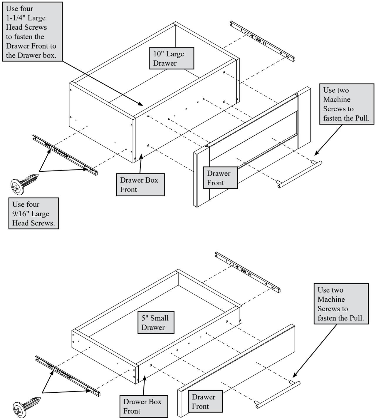
Fasten the Extension Slides to your Drawer box Sides using the 9/16" Large Head screw as shown.
