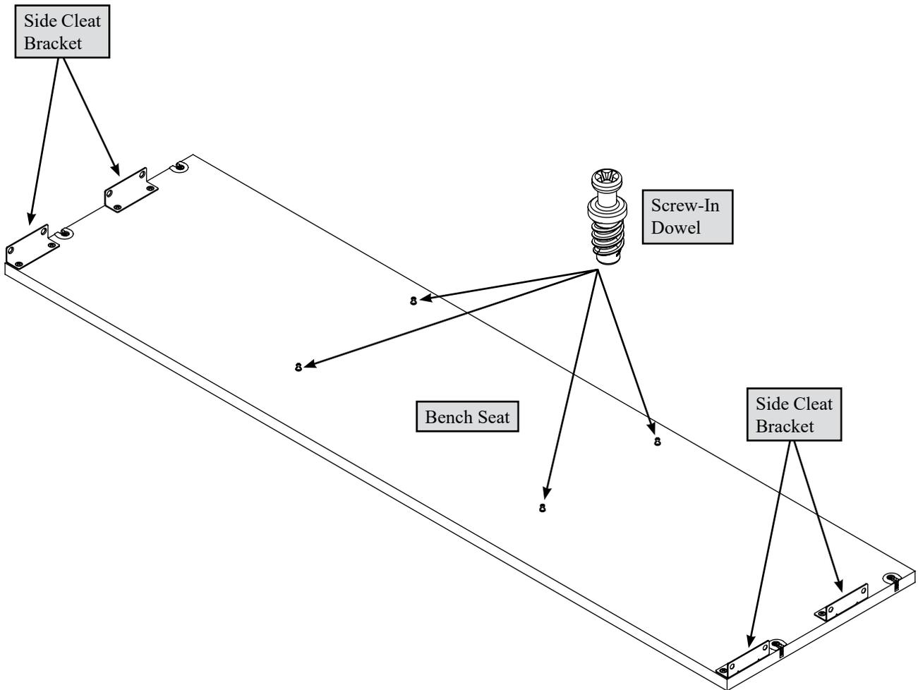
Fasten the Side Cleat Brackets to the Bench Seat with eight 9/16" Wafer Head Screws.
