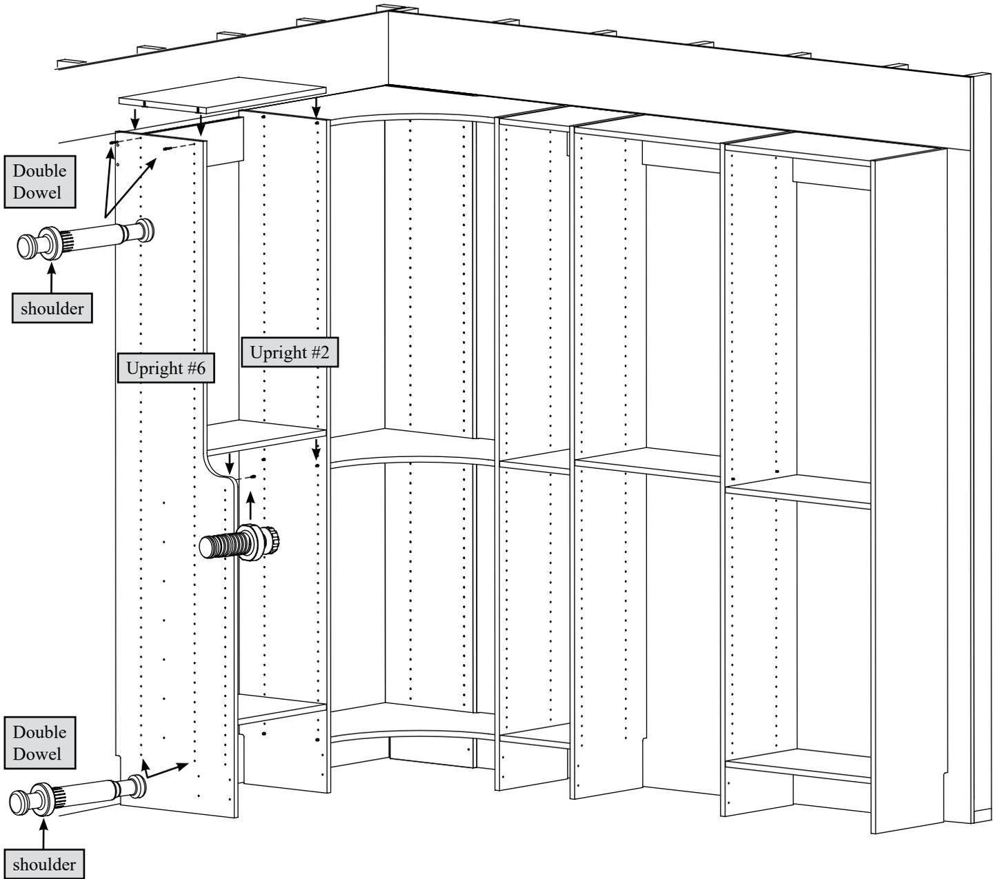
Insert four Double Dowels completely into the holes in Upright #6.
