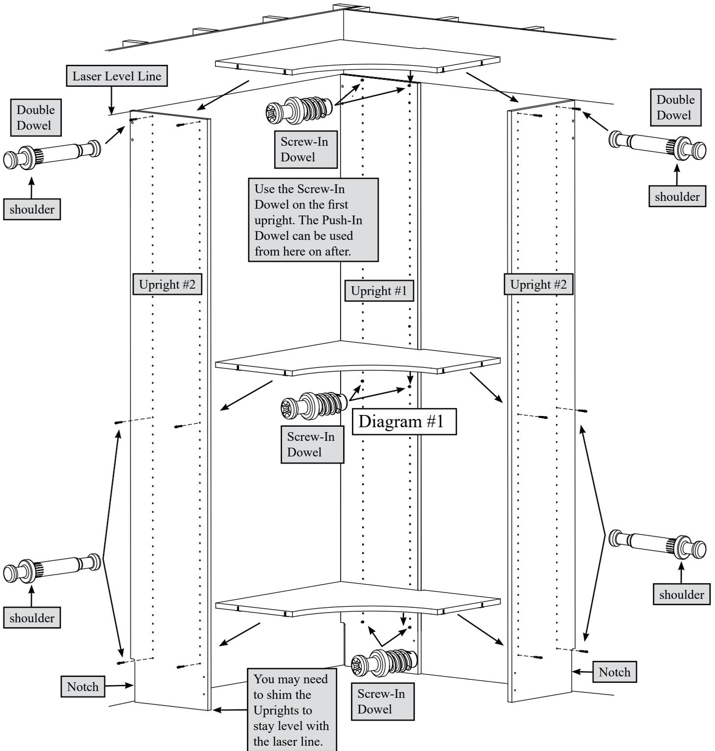
Turn four Screw-in Dowels into the top holes and bottom holes of the corner Upright. Turn additional Screw-In Dowels into the holes per Design in Diagram #1 for placement of the Fixed Shelf.
