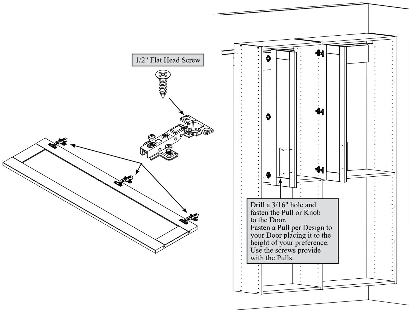
Fasten the Hinges to the Door. Use the Black 1/2" Flat Head Screws.
