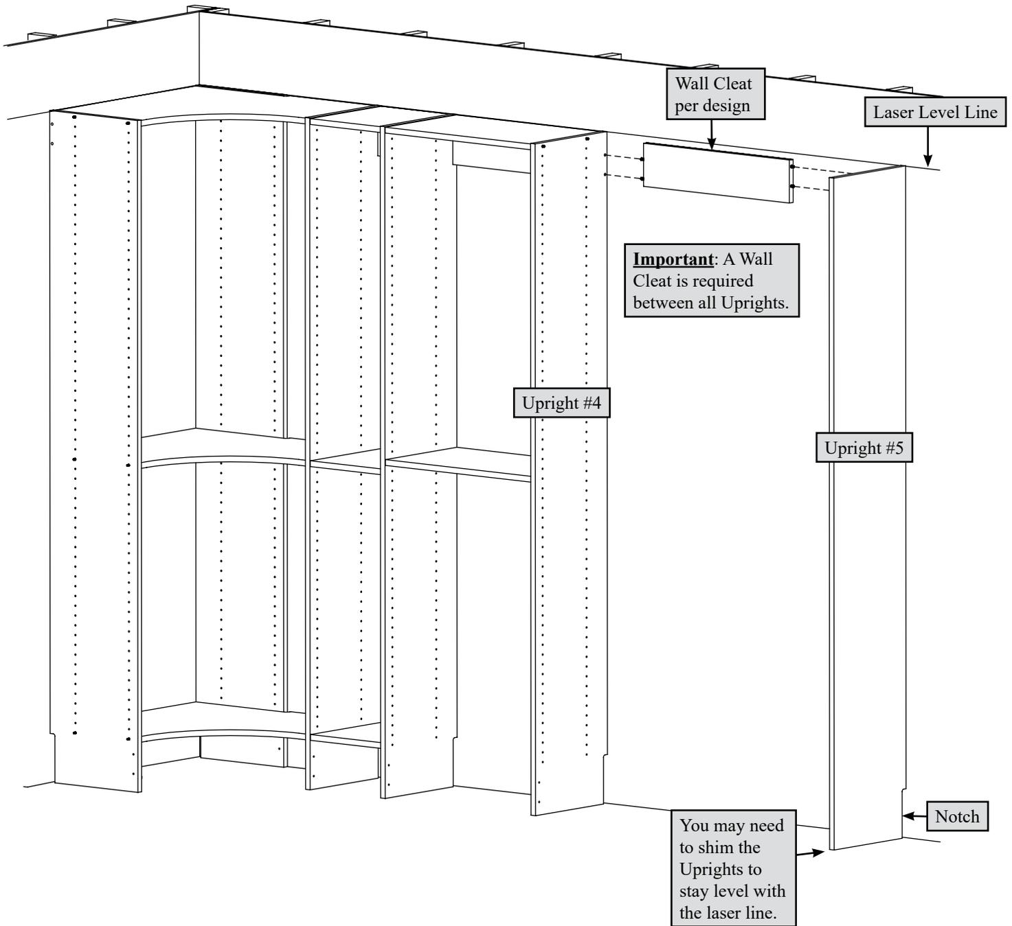
Fasten the Wall Cleat to the Uprights by pushing the wood dowels in the Wall Cleat into Uprights #4 and #5.
