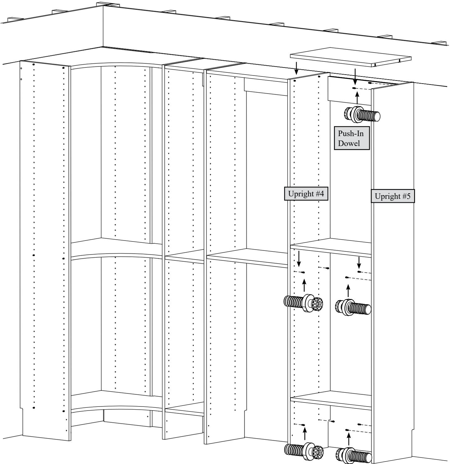
Insert ten Push-In Dowels completely into the holes in Uprights #4 and #5.
