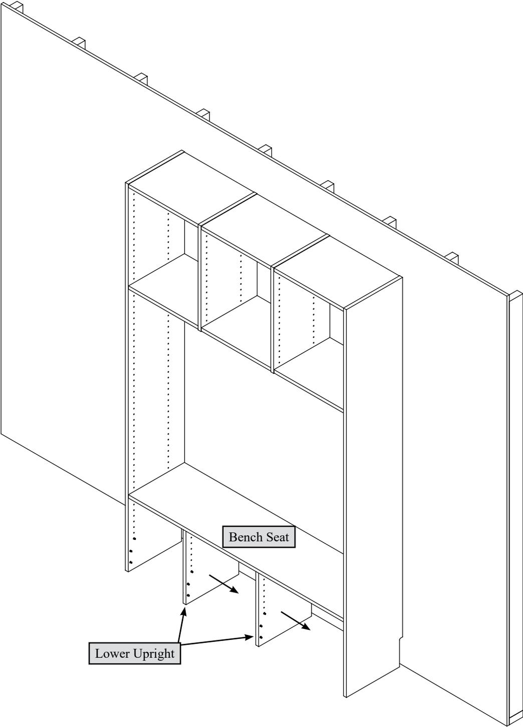
Fasten the Lower Uprights to the Bench Seat. Tighten four Connectors.
