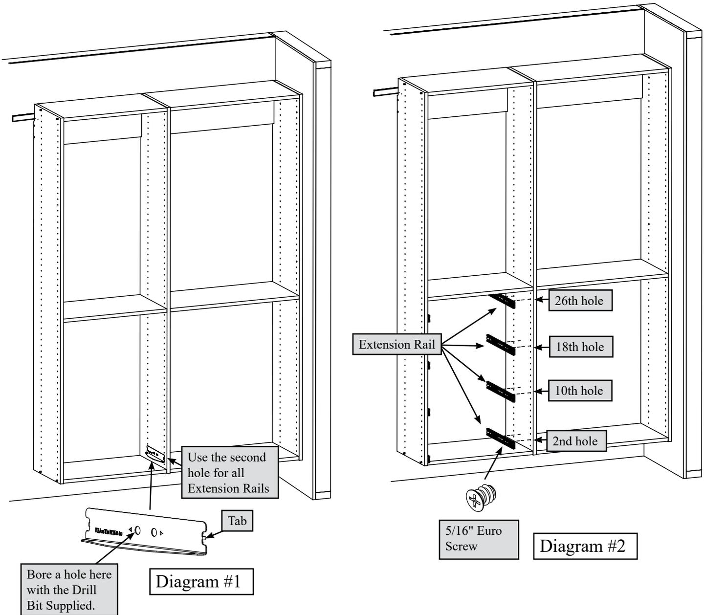
The rear hole for the 350mm Extension Rail requires boring. To do this, insert the tabs on the Rail Template Kit into the proper holes of the Upright. Use the Drill Bit supplied to drill the rear hole in the Template as shown in Diagram #1.
