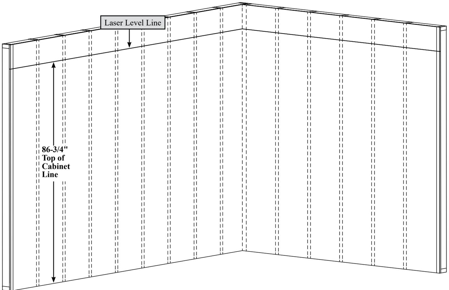
With a level or laser, create a line 86-3/4" off the floor onto your wall to indicate the top edge of the cabinets
