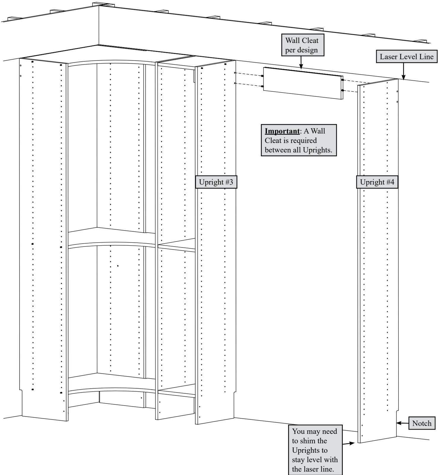
Fasten the Wall Cleat to Uprights #3 and #4 by pushing the wood dowels in the Wall Cleat into the Uprights.
