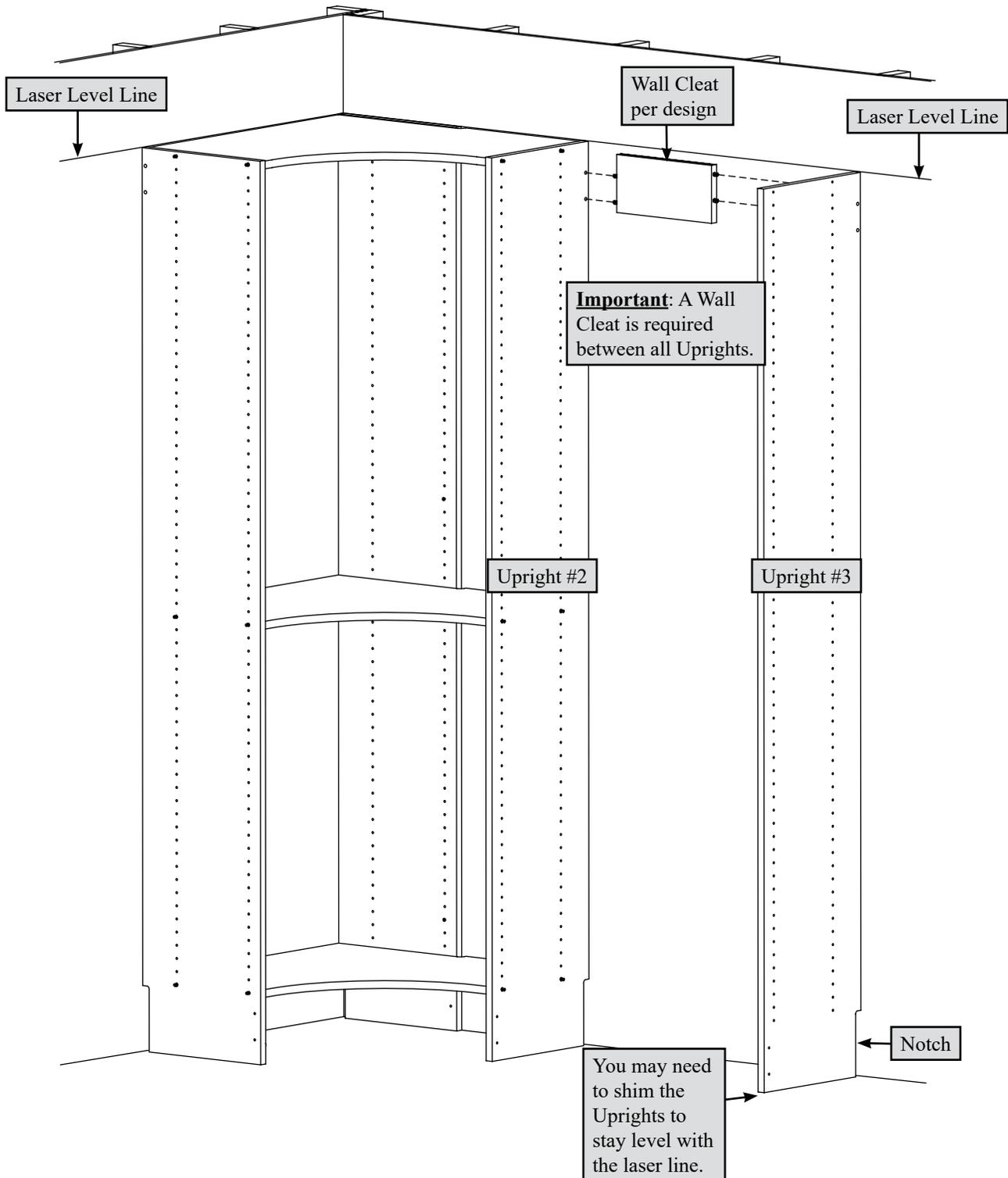
Wall Cleats come with pre-glue dowels in them. Fasten a Wall Cleat to Uprights #2 and #3 by pushing the wood dowels in the Wall Cleat into the Uprights.
