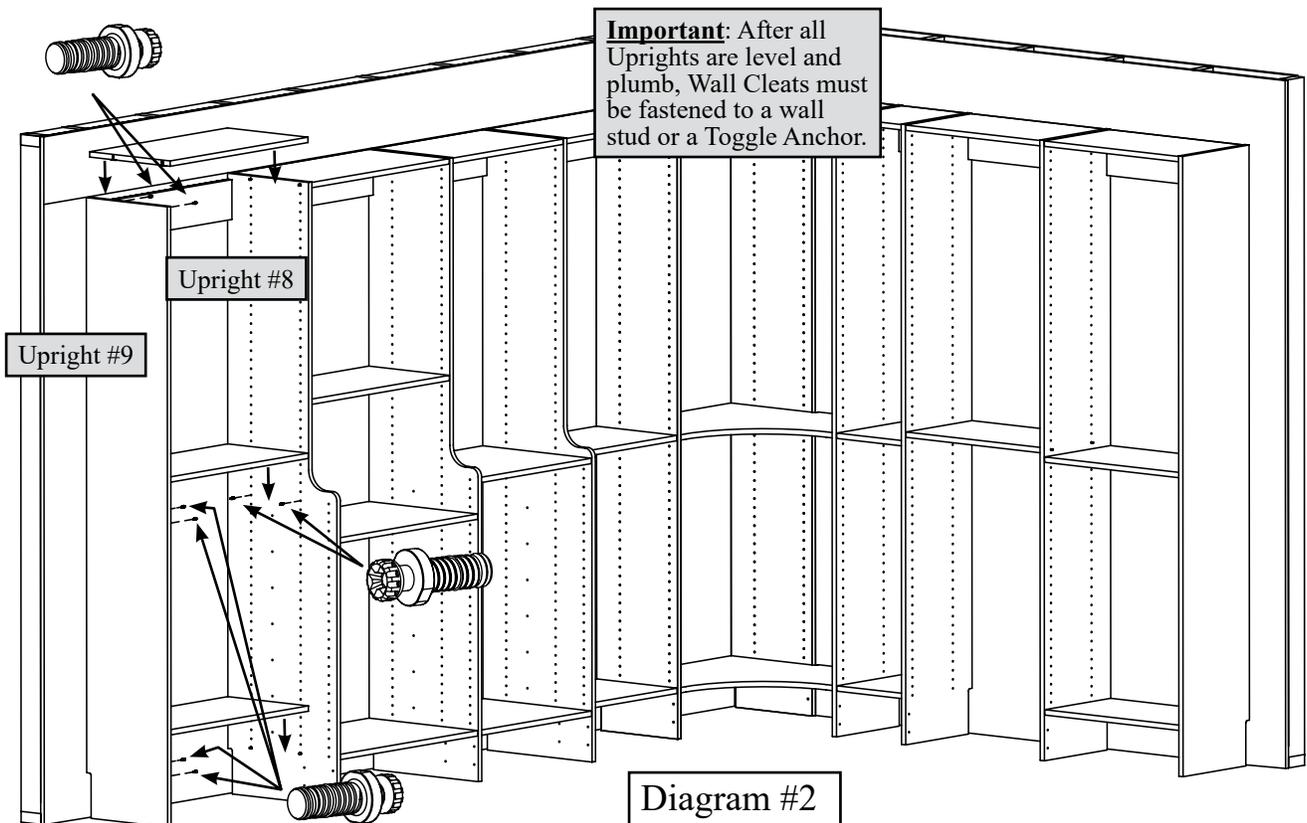
Fasten the Wall Cleat to the Uprights by pushing the wood dowels in the Wall Cleat into Uprights #8 and #9 as shown in Diagram #1. Insert eight Push-In Dowels completely into the holes in Uprights #8 and #9 as shown in Diagram #2. Fasten three Fixed Shelves to Uprights #8 and #9. Tighten twelve Connectors.
