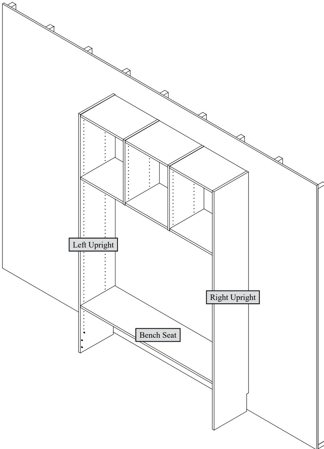
Fasten the Bench Seat to the Left and Right Uprights. Tighten four Connectors.
