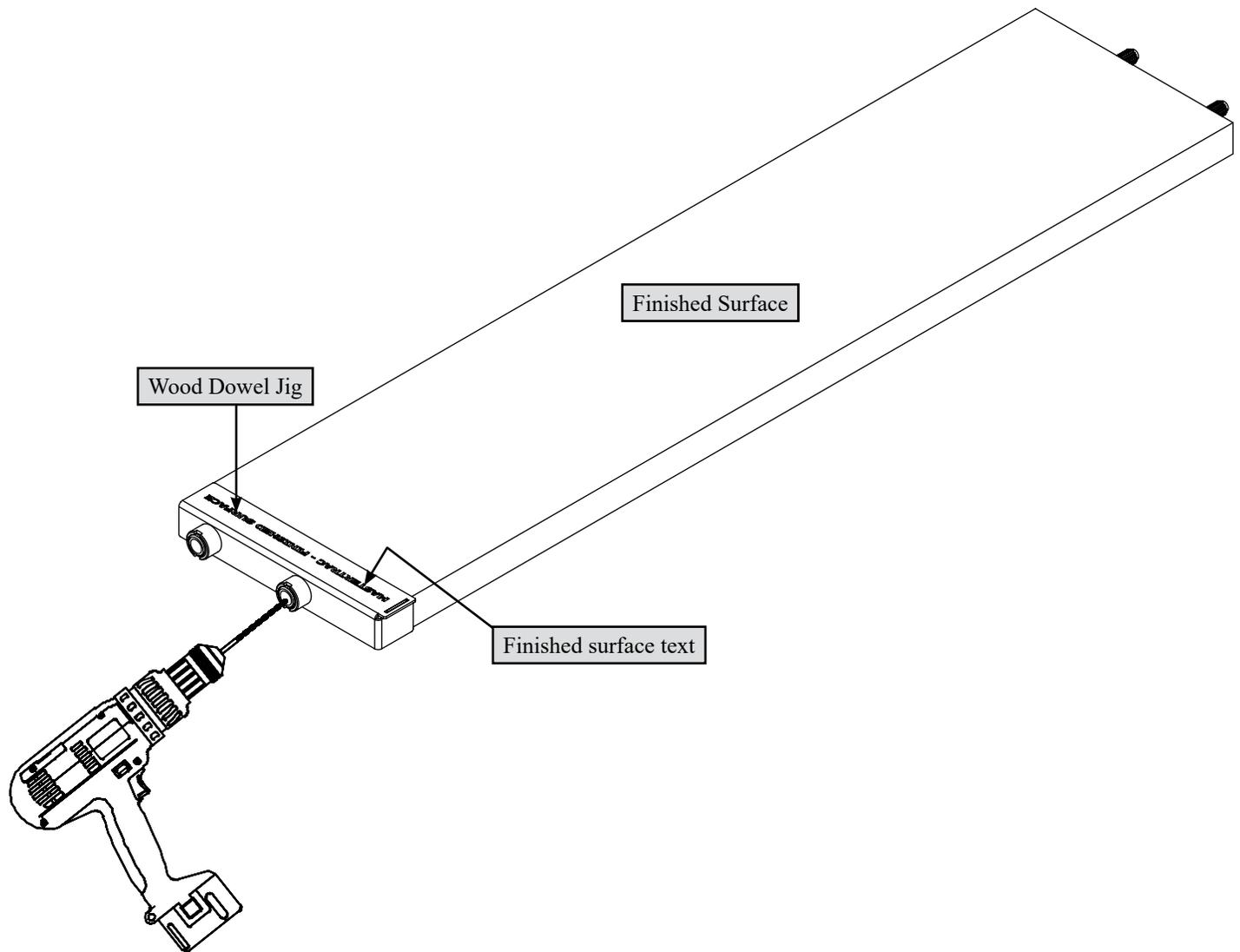
In some Designs, you may need to cut a Cleat to length and rebores holes to replace the Wood Dowels in a Cleat. Follow the diagram and steps below for instructions.
