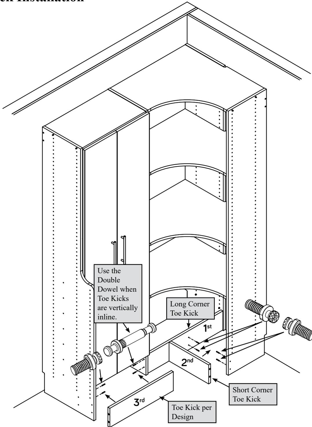
**1<sup>st</sup>** - Corner Floor Cabinets will require a Long Corner Toe Kick and Short Corner Toe Kick. Insert four Push-In Dowels into the right corner Upright against the wall and the left corner upright. Push the connectors in the Long Corner Toe Kick completely onto the upper Push-In Dowels. Next, rotate the Toe Kick on the upper Push-In Dowels until the connectors are exposed. Tighten two upper connectors. Rotate the Toe Kick down completely onto the lower Push-in Dowels.
