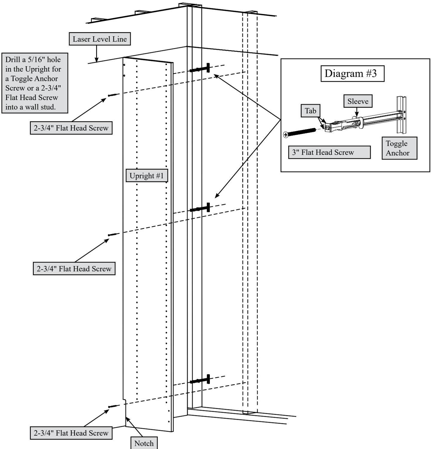
Fasten Upright #1 to the wall with three 2-3/4" Flat Head Screws into wall studs. Use three Toggle Anchors if a wall stud is not available.
