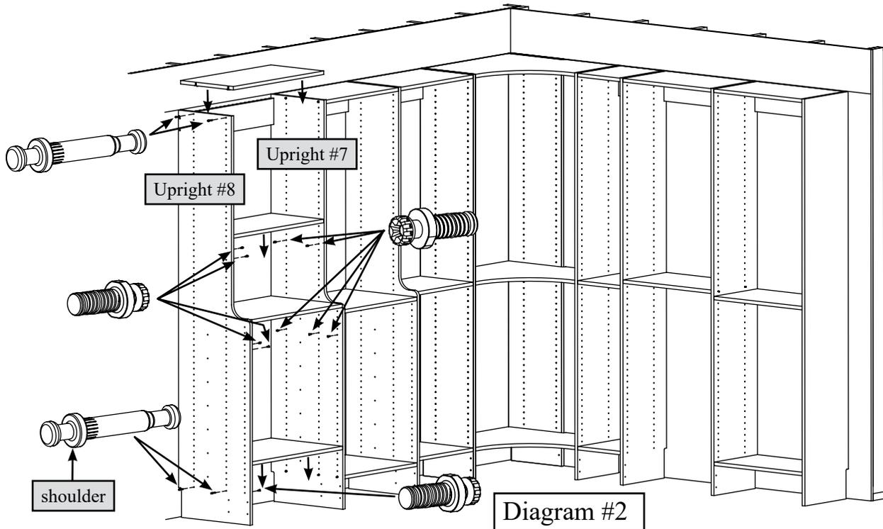
Fasten the Wall Cleat to the Uprights by pushing the wood dowels in the Wall Cleat into Uprights #7 and #8 as shown in Diagram #1.
