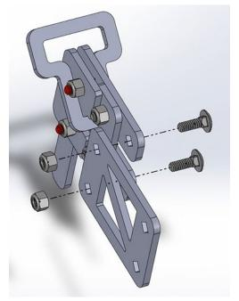
Next, install the side mount sleeves and hook using the provided 4" carriage bolts, as shown. 4" bolts shown in green.
