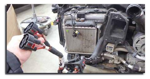
First, you will need a basic understanding of electronics – knowing how to use a DVOM to measure resistance in wires accurately, and the ability to see and chase shorts or damage in literally miles of wires. Learning to read OE specs and understand flow charts will be a must. You'll also need to learn OE requirements on wire repair and options as well as routing and power demands and limitations of circuits.
