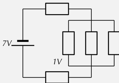
What is the voltage across the parallel resistor combination in the circuit shown?
