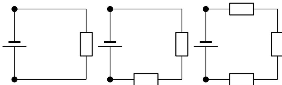
Let us look at this in a bit more detail. In the picture below you can see what the different measurements for 3 identical resistors in series could look like. The total voltage across all three resistors is the sum of the voltages across the individual resistors. Resistors in series are known as voltage dividers because the total voltage across all the resistors is divided amongst the individual resistors.
