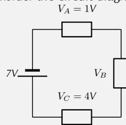
What is the voltage across the unknown resistor in the circuit shown?
