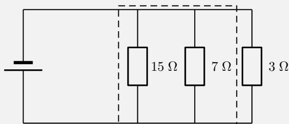
We have already calculated the total resistance of the two resistors in the dashed box to be  $4,77\ \Omega$ . We can replace these two resistors with a single resistor of  $4,77\ \Omega$  to get:
