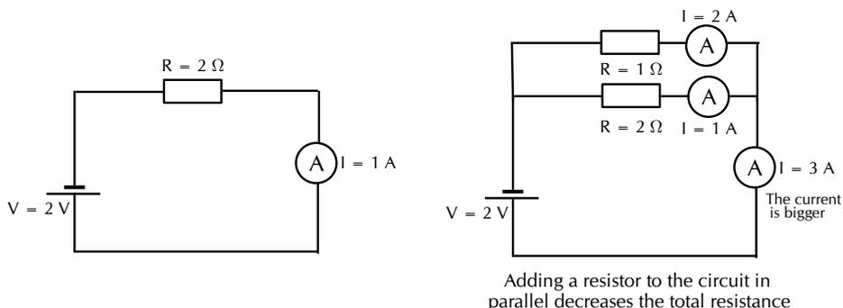
The total resistance of a number of parallel resistors is NOT the sum of the individual resistances as the overall resistance decreases with more paths for the current. The total resistance for parallel resistors is given by:
