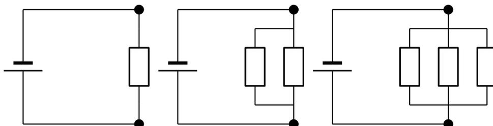
Lets look at two resistors in parallel more closely. When you construct a circuit you use wires and you might think that measuring the voltage in different places on the wires will make a difference. This is not true. The potential difference or voltage measurement will only be different if you measure a different set of components. All points on the wires that have no circuit components between them will give you the same measurements.
