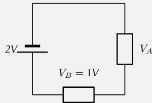
What is the voltage across the unknown resistor in the circuit shown?
