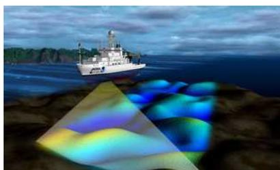
Ships on the ocean make use of the reflecting properties of sound waves to determine the depth of the ocean. A sound wave is transmitted and bounces off the seabed. Because the speed of sound is known and the time lapse between sending and receiving the sound can be measured, the distance from the ship to the bottom of the ocean can be determined. This is called sonar, which is an acronym for **S**ound **N**avigation **A**nd **R**anging.
