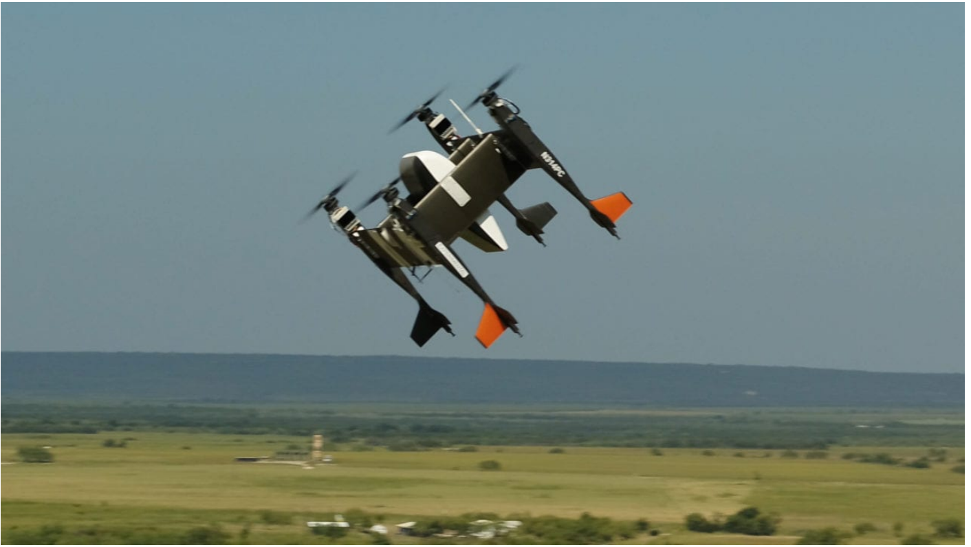
Bell Flight's APT-70 autonomous logistics drone, equipped with Yamato's PUPA-70XG pod, flies above Texas. (Bell Flight)
