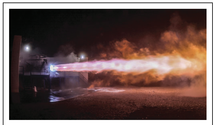
Fig. 21. Raptor engine firing.
