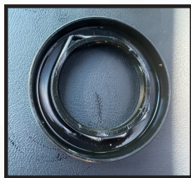
Front and Back of broken shaft seal
