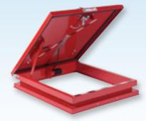
Acralight Solar's Retro-Hatch provides most of the features of a standard Acralight Solar's roof access hatch with a 4" high curb mounted base designed to mount on existing curbs. This design eliminates the expense of removing an existing roof hatch base when performing roof hatch repairs. Standard model provides an extended cap flashing, pre-punched, to receive a safety railing system or AcraGrab safety feature.
