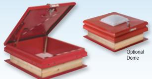
Acralight Solar's galvanized steel or aluminum roof access hatch is designed for safety and reliability. Standard model provides an extended cap flashing, pre-punched to receive a safety railing system or AcraGrab safety feature. Unique cross-broken lid design to eliminate ponding water. Standard 12" high self-flashing curb with wood nailer and a Federal Safety Red high gloss finish. Add an optional SkyTough dome in the lid for natural daylighting in the ladder well.
