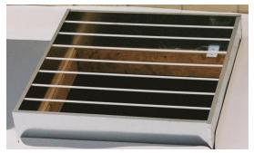
\*Security grilles shall be OSHA and Cal-OSHA compliant. Grilles shall be made of tubular steel .060 thickness and minimum 1/2" diameter. Tubular cross bars shall be welded to1" x 1/8" steel flat strap at minimum 6" OC spacing. For Cal-OSHA compliant grilles a center strap shall be added on all grilles larger than 4x4 size. Center straps shall be punched with tubes running through and welded at every third tube to prevent movement. Complete assembly shall be powder-coated white or galvanized\*
