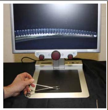
The Inspectis Port is an all-in-one, space-saving, High Definition, The Inspectis Port is a full HD portable inspection system that folds down into a small carry case that allows the technician to travel easily between hospitals, surgery centers and clinics. The unit's 16" or 19" monitor gives enough viewing area to inspect any surgical instrument or kit.
