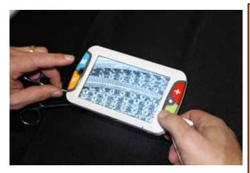
The Inspectis Grip is a handheld, digital inspection system utilizing an HD camera and an integrated, 5" LCD screen for a high quality image. The integrated handle allows the technician greater control and access to the magnification and freeze controls with only one hand.
