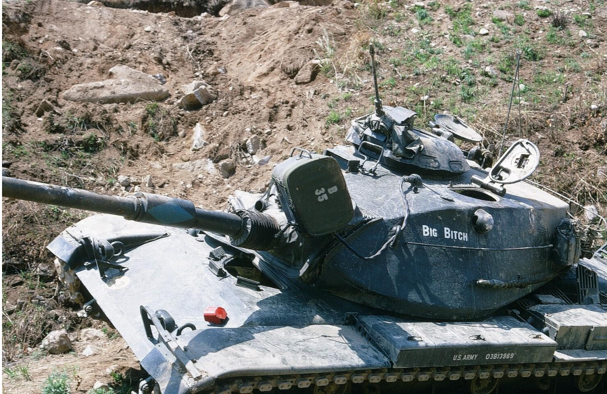
This tank rolled off a hill during night live fire, heavy rain, table 8 gunnery
