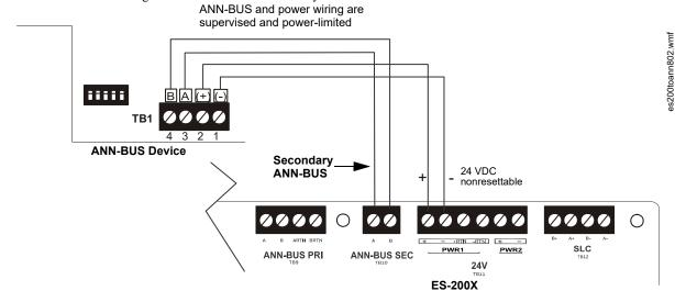
Figure 2.18 illustrates the wiring between the FACP's Secondary ANN-BUS and ANN-BUS devices.
