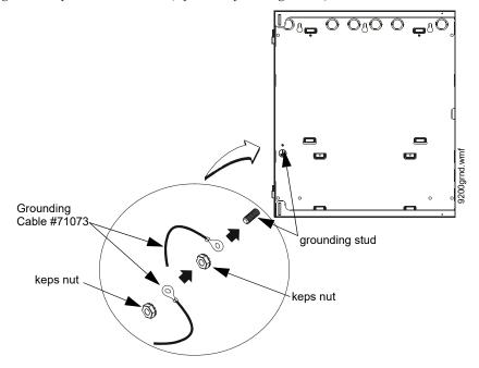
Figure 2.4 Earth Ground Connection
