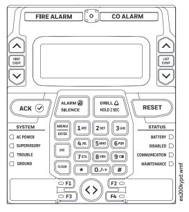
Figure 1.2 Membrane/Display Panel
