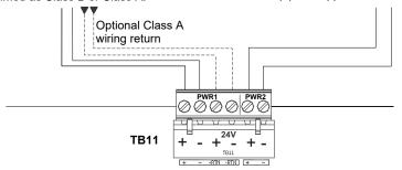
Figure 2.5 Special Application Power Outputs - 24 VDC
