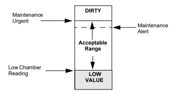
Figure 4.1 Diagram of Maintenance Levels
