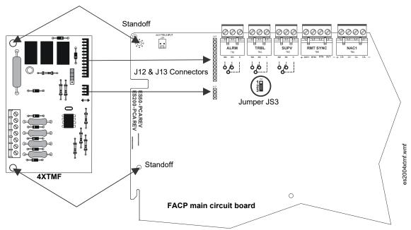
Figure 2.16 4XTMF Connectors to ES-200X Connectors
