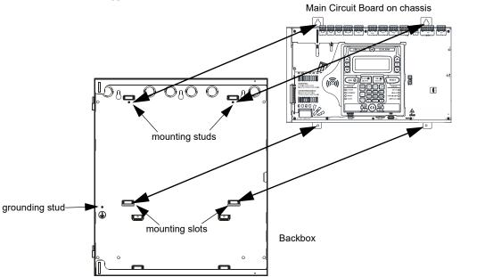
Figure 2.1 ES-200X Chassis Removal and Installation
