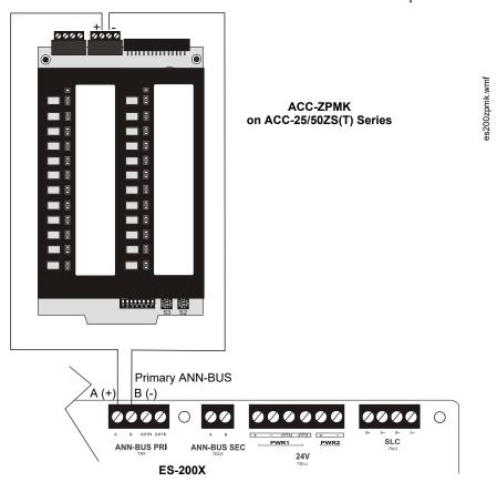
Figure 2.33 FACP Connection to ACC-25/50ZS(T) Series Audio Panel (Legacy)
