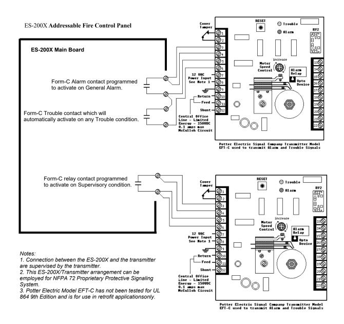
Figure C.3 Proprietary Protective Signaling System
