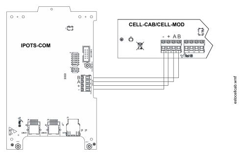
Figure 2.14 Wiring the CELL-CAB/CELL-MOD
