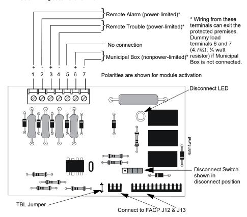
Figure 2.15 4XTMF Transmitter Module
