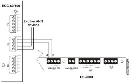
Figure 2.32 FACP Connection to ECC-50/100 Series Audio Panel
