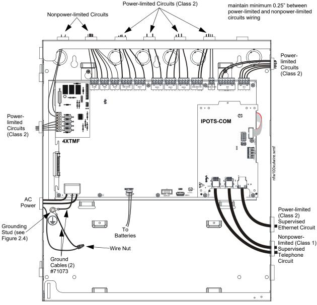
Figure 2.10 Typical UL Power-limited Wiring Requirements
