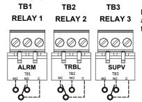
Relay contacts shown <u>with</u> power applied to panel and no active troubles, alarms or supervisories
