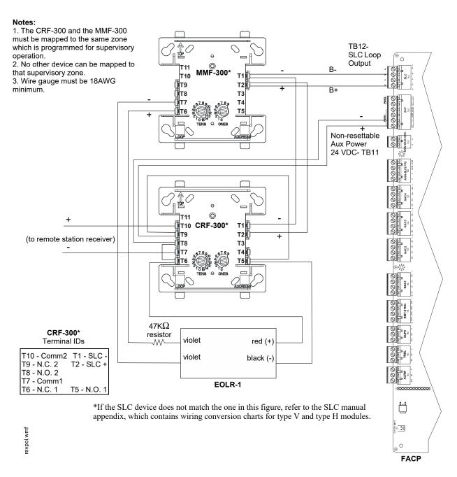
Figure J.3 Alternate Transmission for Supervisory Signals
