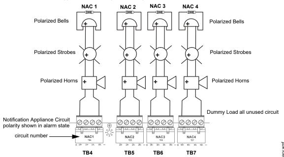
Figure 2.7 NAC Class B Wiring
