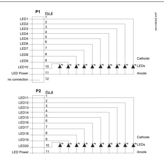
Figure 2.24 ANN-I/O LED Wiring
