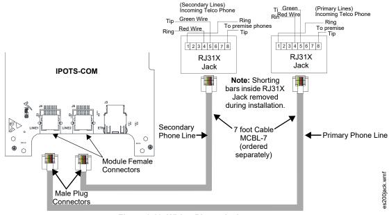
Figure 2.12 Wiring Phone Jacks
