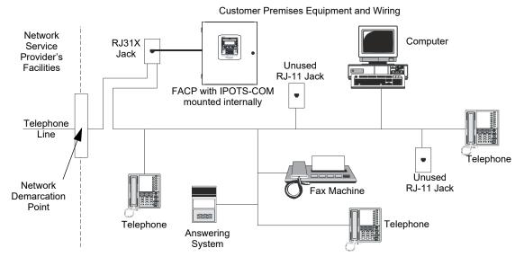
Figure 2.11 Communicator Installation
