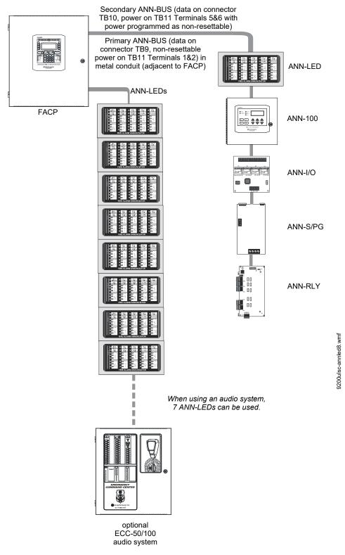
Figure J.2 FACP Maximum Configuration - Eight ANN-LEDs
