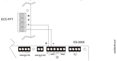
Figure 2.30 ECC-FFT Connections
