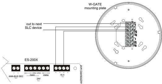
Figure 2.31 W-GATE SLC Connection
