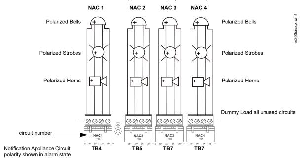
Figure 2.8 NAC Class A Wiring
