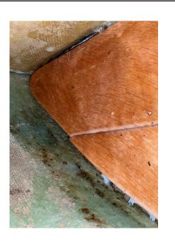
These are " 4" DPI Screw-Down Deckplates" and were \$10 each. These are from Duckworks Boat Builder Supply in Gig Harbor, WA. On these deckplates the lid covers the screw holes, which leaves a clean look on the boat. Other models leave the screws visible when the hatch is closed.
