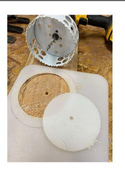
Using the gasket ring you just made as a template, mark the area that will be the mating surface between the gasket ring and the seat. If you use the same deckplate I did, then that outer diameter will be exactly 6".
