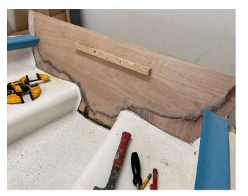
Before installing the wood, I completely sealed it in West System epoxy. I was especially careful to put extra coats around the edges of the wood and on the part that will be behind the seats.
