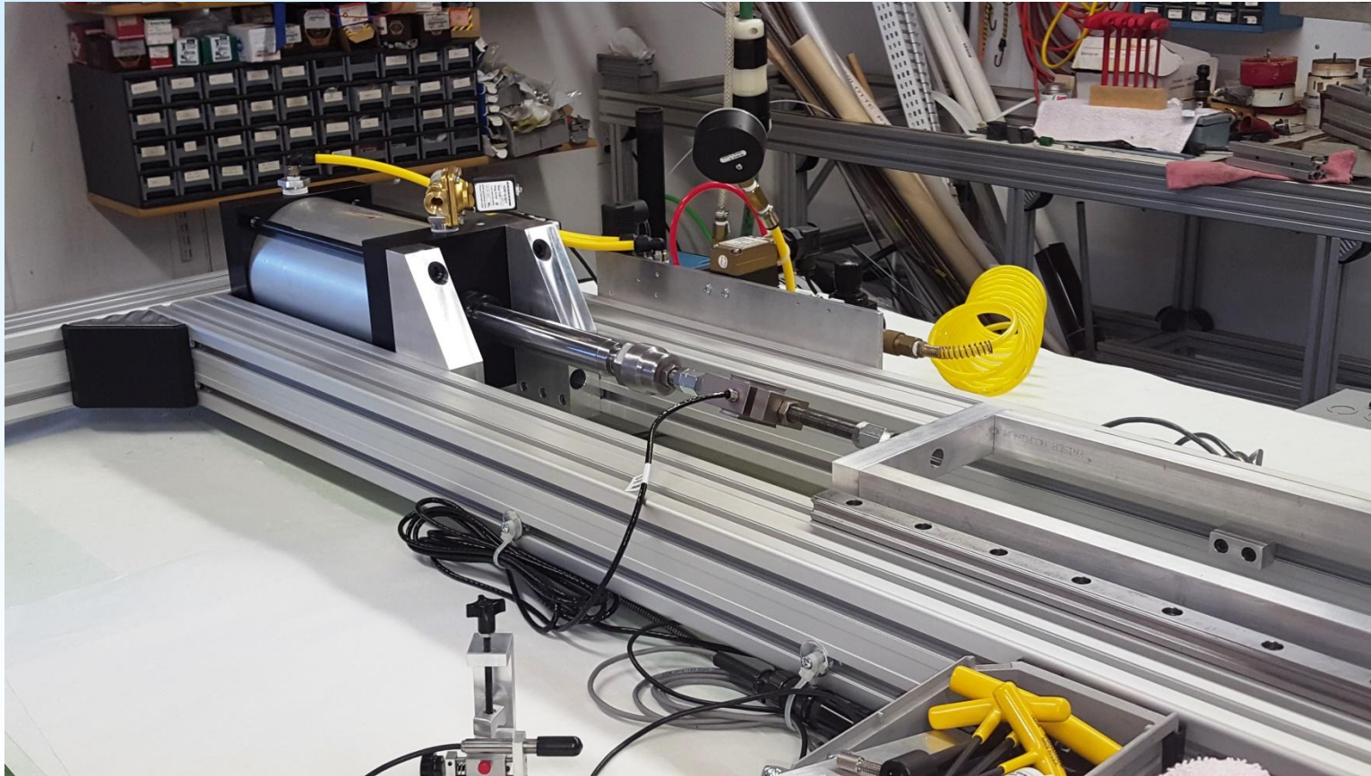
Pneumatic cylinder, load cell and yoke
