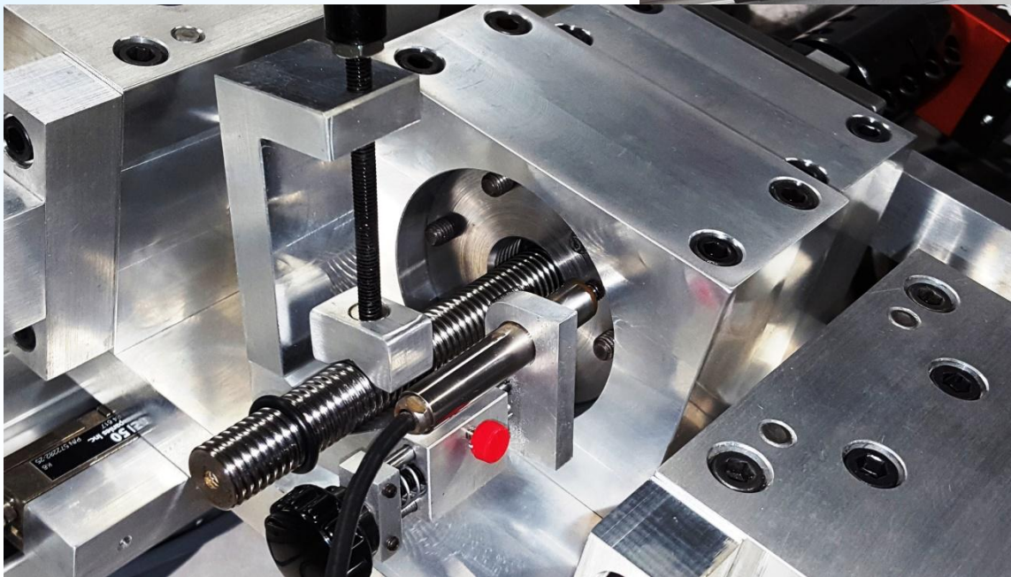
LVDT and holder staged on screw to measure displacement of nut block
