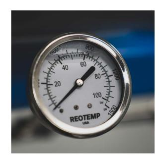
All systems come equipped with 2-1/2" stainless steel pressure gauges with a dual scale 0 - 1,500 psi / 0 - 100 bar pressure rating.
