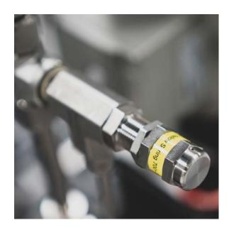
Safety comes first; each dosing pump includes pressure relief valves with a cracking pressure range from 750 –1500 psig and a maximum working pressure of 6000 psig @ 68°F.
