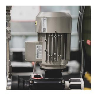
The EMEC pumps used on all Anodamine systems come standard with industry-trusted Siemens SIMOTICS motors (3~Mot. 1AV1073B D-90441)
