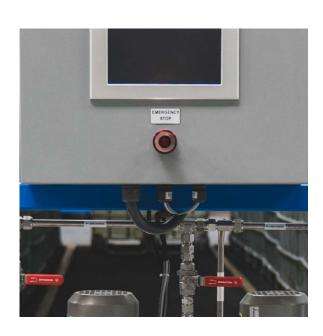
At the push of a button, an emergency stop effectively disconnects power to the entire system. Conveniently located front and center on the system, the user has easy access at all times during operation.
