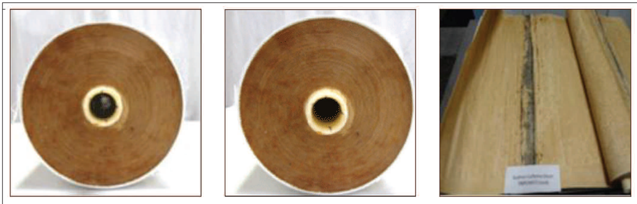
Figure 2: Feed scroll end (left), concentrate scroll end (center), and exposed membrane surface (right) of membrane removed September 2011.
