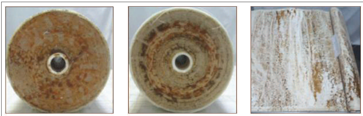
Figure 3: Feed scroll end (left), concentrate scroll end (center), and exposed membrane surface (right) of membrane removed April 2013.
