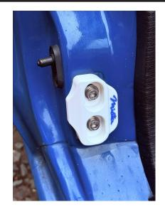
Unscrew and take out the factory door bushing from the door frame.
