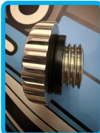
The 2mm shim will flip the cap 180 degrees the 1mm shim 90 degrees and the 0.50mm will allow minor adjustments please fit the shims towards the top on the rubber seal and not directly to the cam cover
