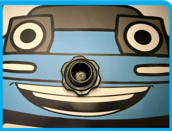
First, remove the old oil seal from the original cap. Use a fine-tipped tool to do this, and slowly work the seal upward towards the end of the cap.
