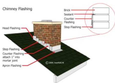
Typical chimney flashing
