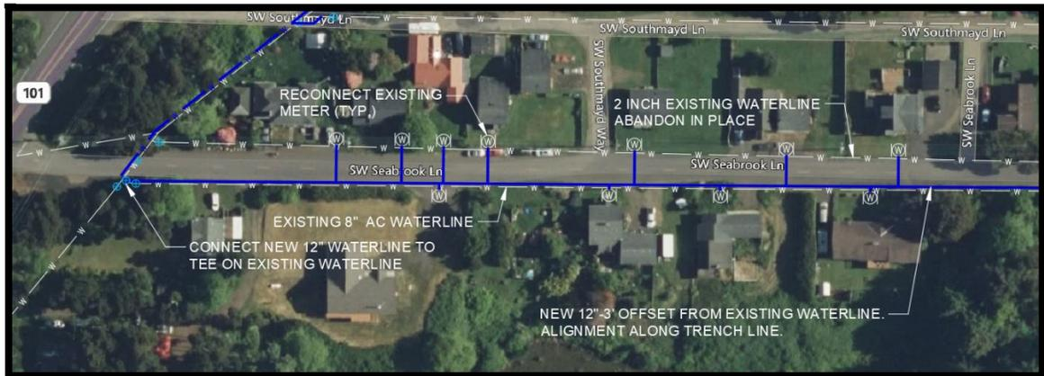
**Figure 1A - Seabrook Lane Waterline Improvement Layout (West End)**
