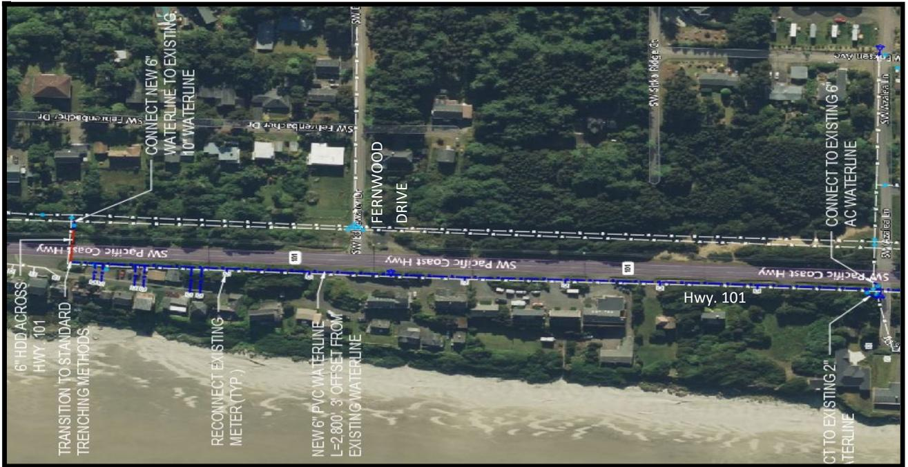
**Figure 6 - W. Side of Hwy. 101 Waterline Site Improvement Layout (North Section)**
