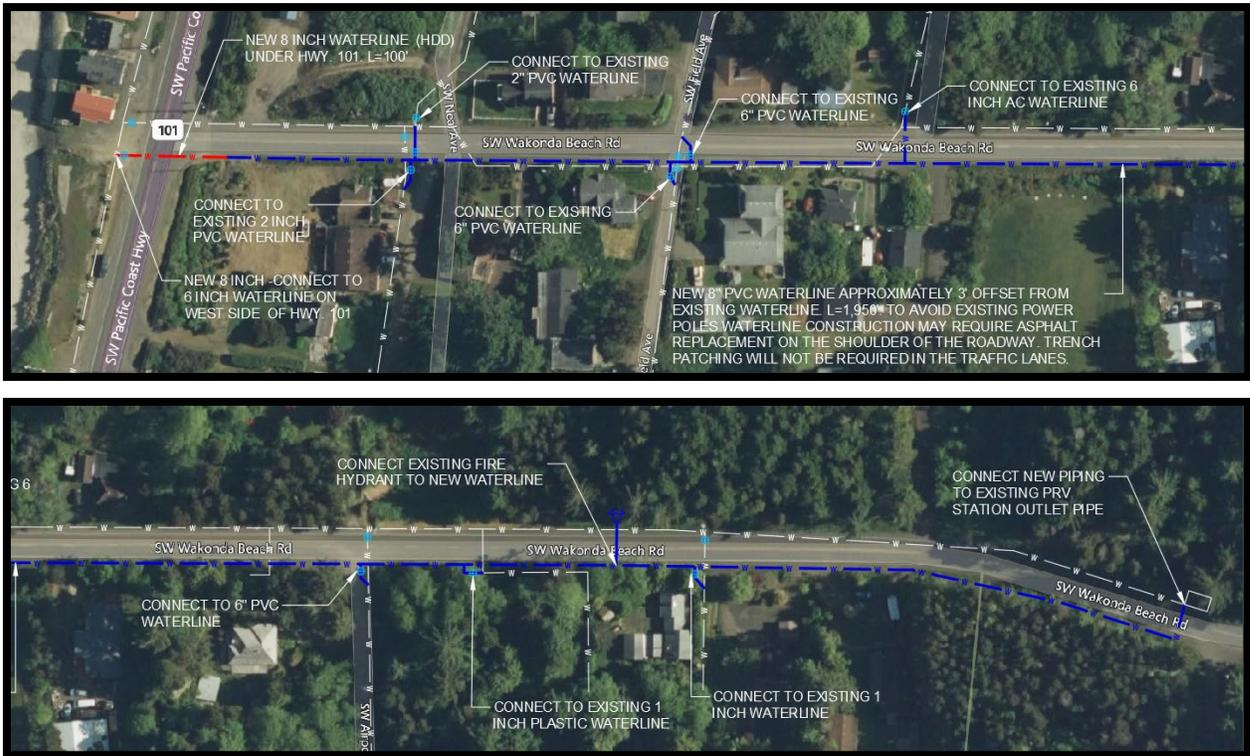
**Figure 2 - SW Wakonda Rd. Waterline Project Layout**
