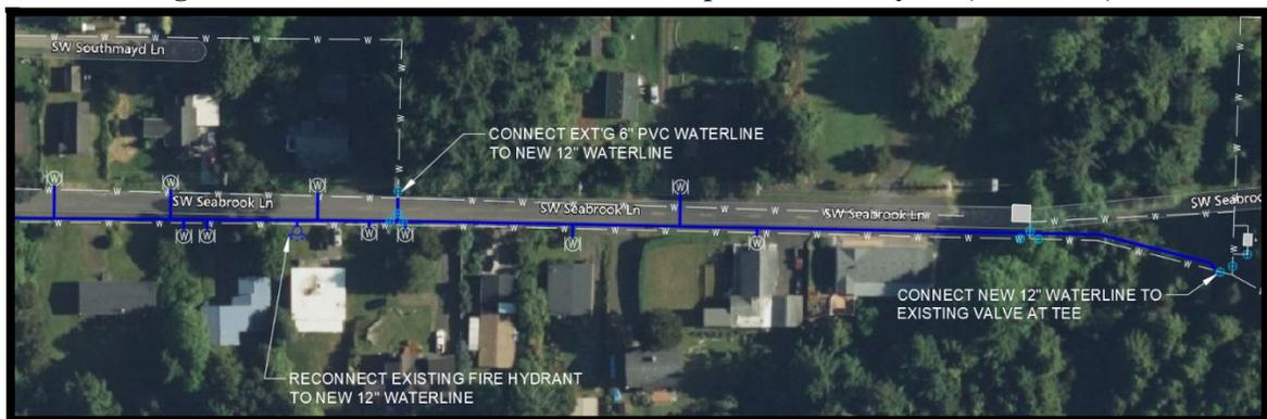
**Figure 1B - Seabrook Lane Waterline Improvement Layout (East End)**
