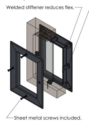
Threaded nut accepts sheet metal screw, positions glass in the door cutout & provides tamper-resistance from corridor side.
