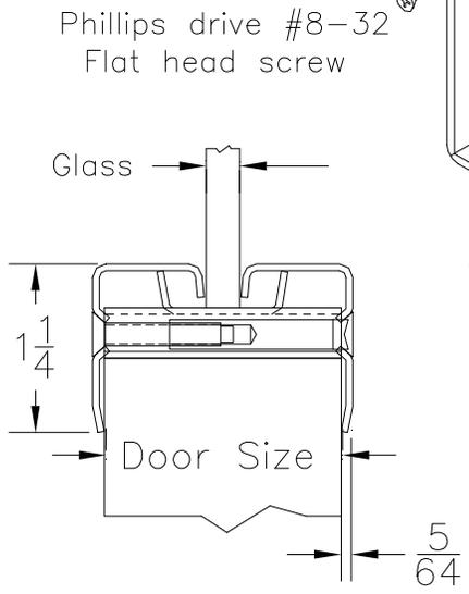
**NOTE ON GLAZING TAPE:** Some types of glass & some very large frames require glazing tape. Scan the QR Code (right) or visit [www.allmetalstamping.com](http://www.allmetalstamping.com) for a listing of approved glazing, fire ratings, or additional installation requirements such as tape or intumescent.
