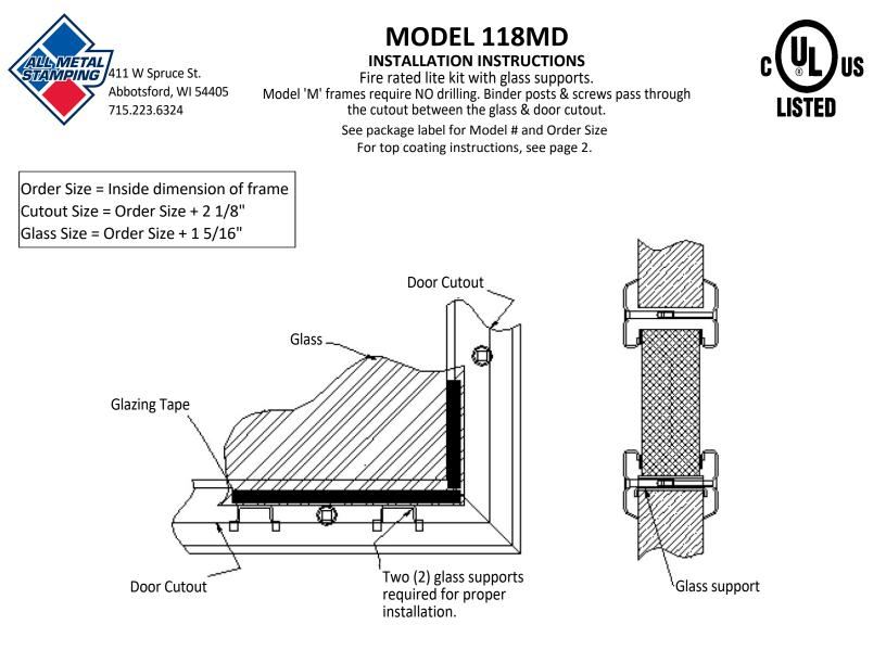
**NOTE ON GLAZING TAPE:** Some types of glass & some very large frames require glazing tape. Scan the QR Code (right) or visit www.allmetalstamping.com for a listing of approved glazing, fire ratings, and glazing tape requirements.
