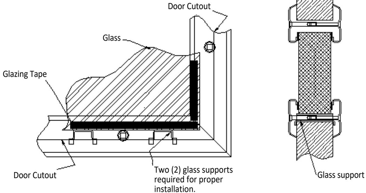
**NOTE ON GLAZING TAPE:** Some types of glass & some very large frames require glazing tape. Scan the QR Code (right) or visit [www.allmetalstamping.com](http://www.allmetalstamping.com) for a listing of approved glazing, fire ratings, and glazing tape requirements.
