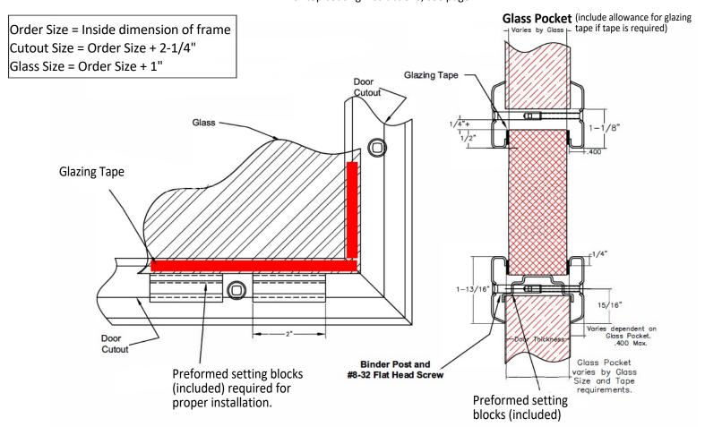
**NOTE ON GLAZING TAPE:** Some types of glass & some very large frames require glazing tape. Scan the QR Code (right) or visit www.allmetalstamping.com for a listing of approved glazing, fire ratings, and glazing tape requirements.
