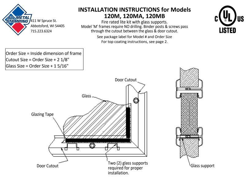
**NOTE ON GLAZING TAPE:** Some types of glass & some very large frames require glazing tape. Scan the QR Code (right) or visit *www.allmetalstamping.com* for a listing of approved glazing, fire ratings, and glazing tape requirements.
