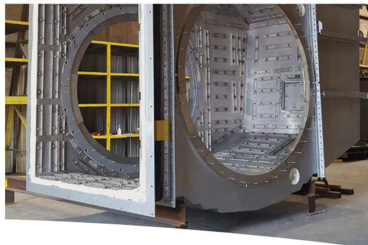
Complete assembly of a FS7EA exhaust plenum.
