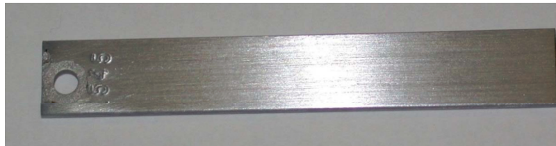
TYPICAL MILD STEEL CORROSION – 1.5 MPY
