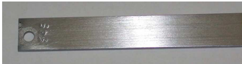
TYPICAL MILD STEEL CORROSION – 0.27 MPY
