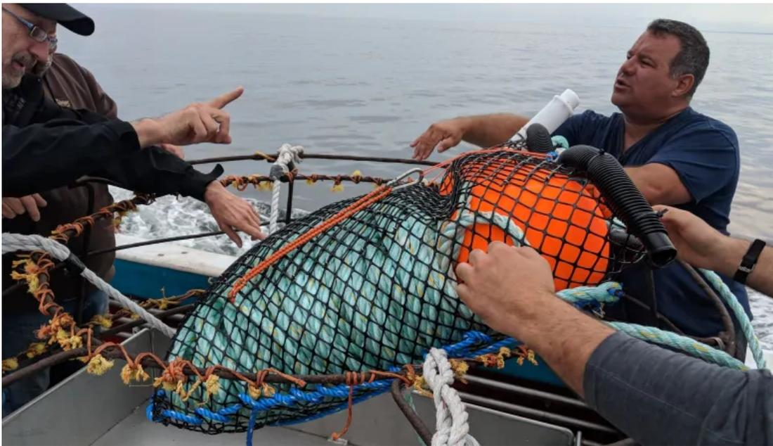
Fishermen in Caraquet test traps that have bags attached to them. The bag holds the rope needed to pull the trap up. An acoustic release device triggers the rope when the fishermen are ready to pull the trap from the ocean floor. (Marco Flagg/Submitted)
