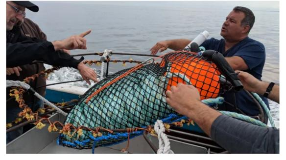
Fishermen in Caraquet test traps that have bags attached to them. The bag holds the rope needed to pull the trap up. An acoustic release device triggers the rope when the fishermen are ready to pull the trap from the ocean floor. (Marco Flagg/Submitted)
