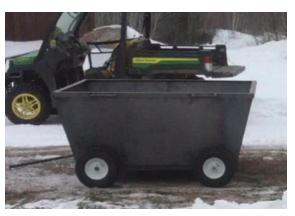
For kiln #2 - a handle/hitch for pulling the kiln with welded axels and removeable wheels.
