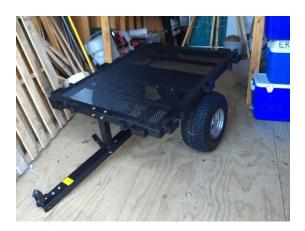
For Kiln #1 - a heavy duty lawn cart to carry a kiln pulled by light equipment
