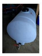
A 65 gallon water tank our experts indicated would be adequate for quenching the kiln contents to stop the pyrolysis process before reaching the ash stage. The tank was fitted with a valve to accept a standard garden hose and would use gravity flow with the tank elevated above the kiln to produce water flow.
