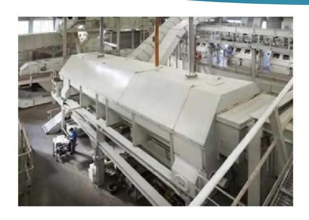
Naste moves into the Mechanical-Biological Waste Treatment Plant for decomposition and fermentation to increase the caloric value of the waste by up to 50%.
