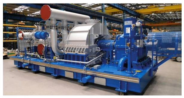
The gas engine waste heat is fed into a steam turbine system producing up to 35% additional electricity.
