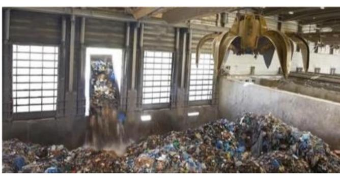
▶ Waste is deposited into a closed bunker.
