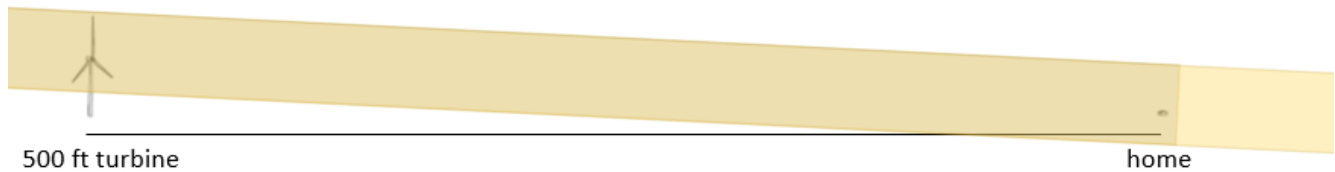
Figure 1: Shadow Flicker For a Typical 500-ft Tall Turbine is 1722 meters (5649.6 ft), which is equal to 11.3:1 distance-to-height ratio.
