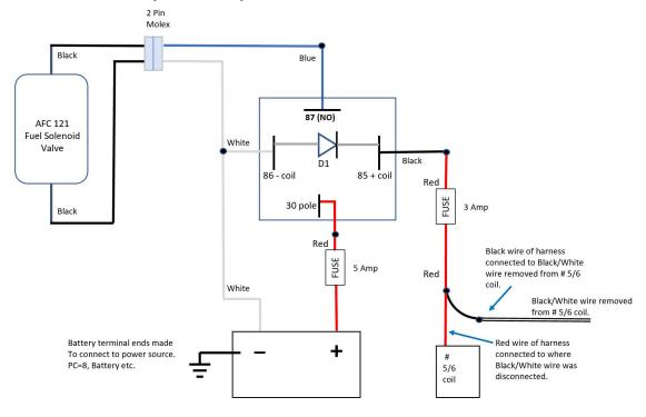
We are using the "safety circuit" 12 V Coil Black/White wire connection to trigger the relay. When the key is turned on, if the safety circuit is satisfied, 12 V is supplied to 85 of the relay, which energizes the relay. The relay then routes power from the battery through 30, to 87 of the relay, and energizes the
