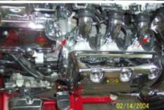
View of the air feed pipe going to exhaust port 3 under the engine on the right hand side.
