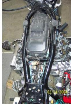
Remove the PAIR control valve assembly and also the 2 attached vacuum tubes going to intakes 3 and 4.
