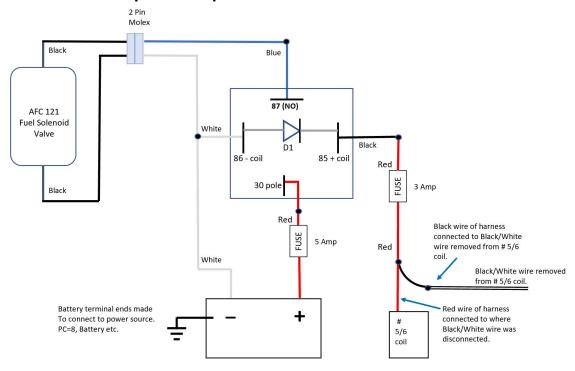
We are using the "safety circuit" 12 V Coil Black/White wire connection to trigger the relay. When the key is turned on, if the safety circuit is satisfied, 12 V is supplied to 85 of the relay, which energizes the relay. The relay then routes power from the battery through 30, to 87 of the relay, and energizes the fuel solenoid. The fuel solenoid will remain energized until any shutoff signal is received. The safety
