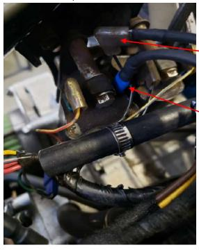
Black/White wire connector disconnected from #5 coil and connected to Black wire from relay harness marked "To B/W wire from #5 coil."
