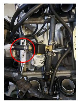
NOTE: fuel lines are not yet connected to fuel rail nipples in this picture. Leave them disconnected at this time. They will be installed in step 32.
