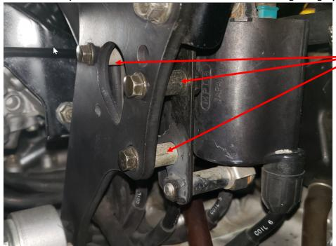
The coils are mounted on a plate with a spacer collar on each 6mm bolt.
