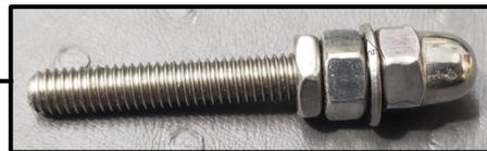
7. Hold the thick nut with a 10mm wrench and tighten the thin nut as a jamb nut against the thick nut.
