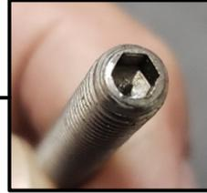
2. On the hex drive end of the stud, install a 6mm thin nut about 5/8 to 3/4 inch onto the stud.
