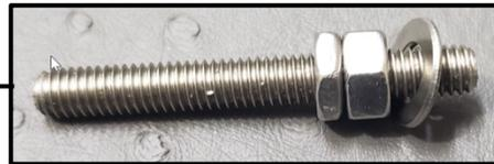
5. Install (1) 6mm cap nut. Adjust the thin nut, thick nut, and washer so that the cap nut is screwed all the way down onto the stud. Snug the washer, thick nut, and thin nut against the cap nut.
