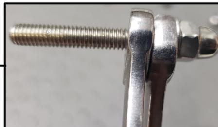
8. Remove the cap nut and washer.
