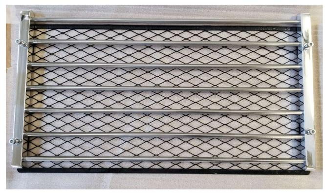
NOTE: The screw holes in the grill match the screen, however the holes in the radiator sides move with the sides and the clip nuts.
