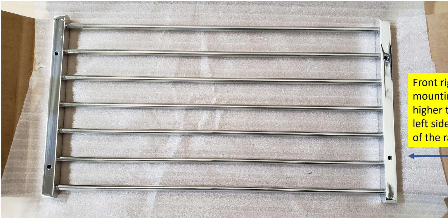
Front right lower mounting hole is higher than the left side hole because of the radiator hose.
