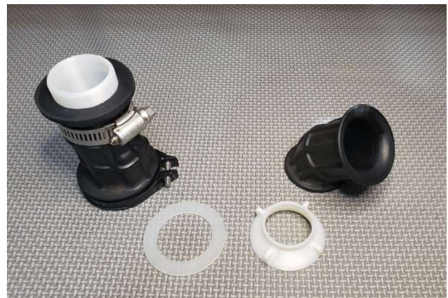
Completed airbox mod tube with washer, nut, and venturi.
