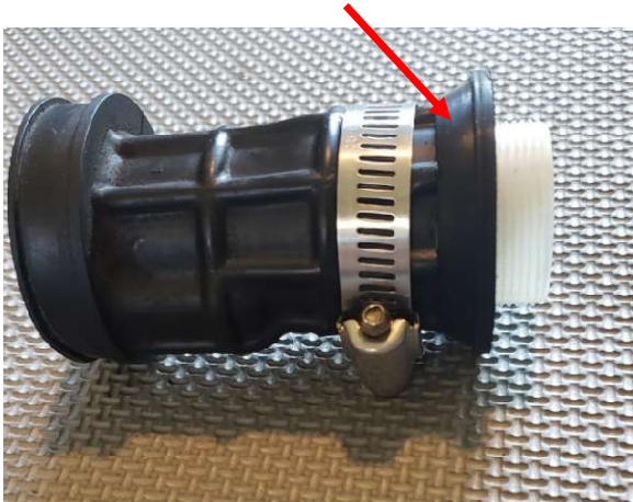
Completed airbox mod tube.
